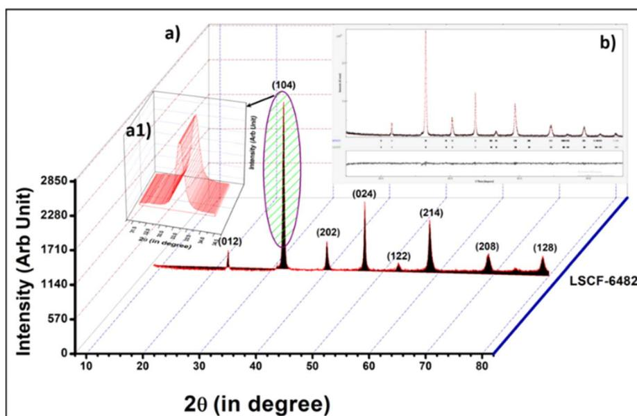
Fig. 10 (a) X-ray diffractogram of LSCF6482 along with the (a1) inset of peak with 100% peak intensity. (b) Rietveld refinement for XRD of LSCF6482.
