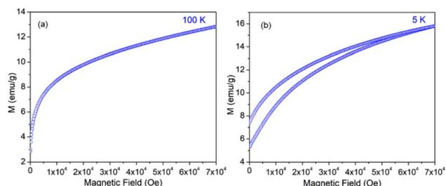
Fig. 2 MH loop for LSCF6482 at: (a) 100 K and (b) 5 K temperature.
