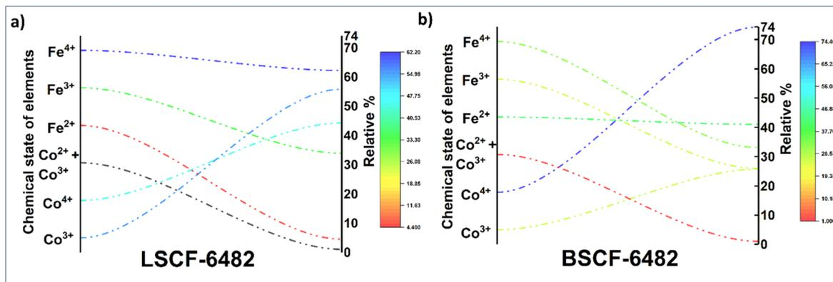
Fig. 5 Relative population of ions with variable oxidation states calculated from XPS analyses of: (a) LSCF6482 and (b) BSCF6482.
