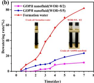
Fig. 9 (a) Crude oil and various types of emulsion viscosity testing and (b) stability evaluation.
