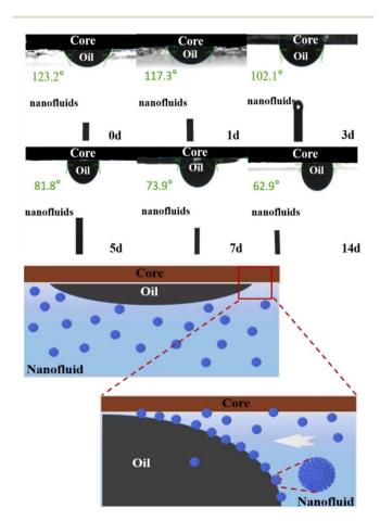
**Fig. 6** Three-phase contact angles of rock surface treated by 300 ppm of GOPH nanofluids.
