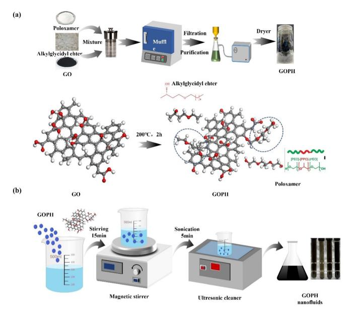
ig. 1 Schematic diagram of the synthetic route of GOPH (a) and process diagram of preparation of GOPH nanofluids (b).
