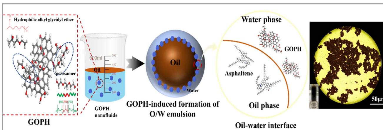
Fig. 11 Mechanism of GOPH-induced formation of viscosity-reducing emulsions in crude oil.
