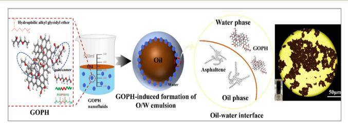
Fig. 11 Mechanism of GOPH-induced formation of viscosity-reducing emulsions in crude oil.
