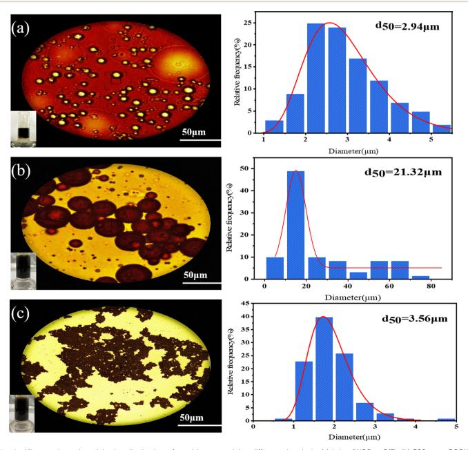
Fig. 8 Micrographs and particle size distribution of emulsions containing different chemicals: (a) brine (WOR = 5/5); (b) 300 ppm GOPH nanofluids (WOR = 8/2).
