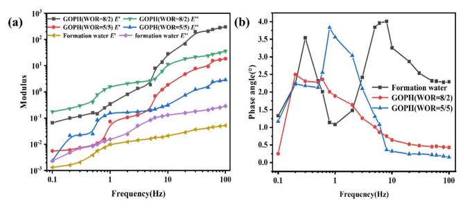
Fig. 10 Interfacial expansion modulus (a) and phase angle of various types of emulsions (b).
