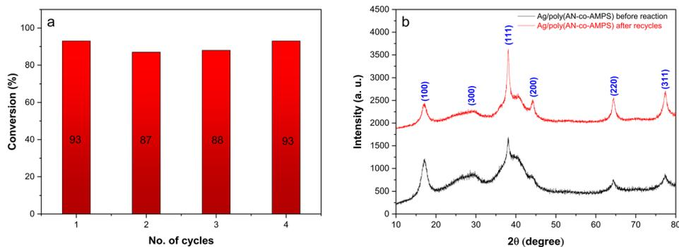
Fig. 11 (a) Recycling experiments for the catalytic reduction of 4-NP to 4-AP. Reaction conditions: [4-NP] = 0.1 mM, [NaBH<sub>4</sub>] = 10 mM, weight of catalyst Ag/poly(AN-co-AMPS) = 20 mg and time = 12 min; (b) XRD analysis of Ag/poly(AN-co-AMPS) before and after the recycling experiments.
