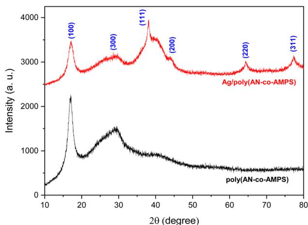
Fig. 4 XRD patterns of poly(AN-co-AMPS) and Ag/poly(AN-co-AMPS).
