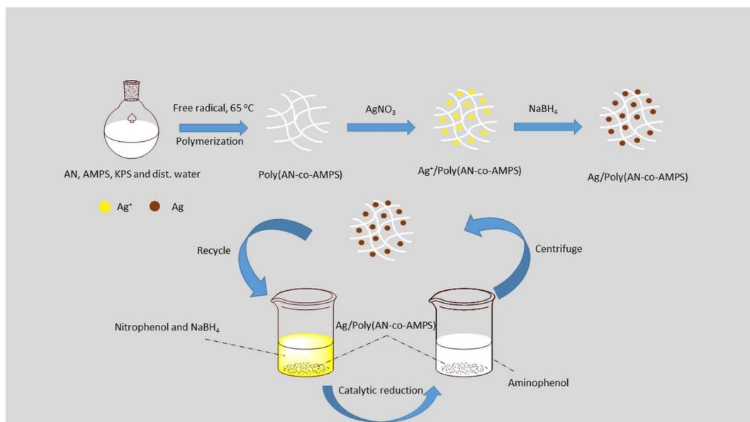
Fig. 1 Synthesis of Ag/poly(AN-*co*-AMPS) as a heterogeneous catalyst for the catalytic reduction of 4-nitrophenol to 4-aminophenol.
