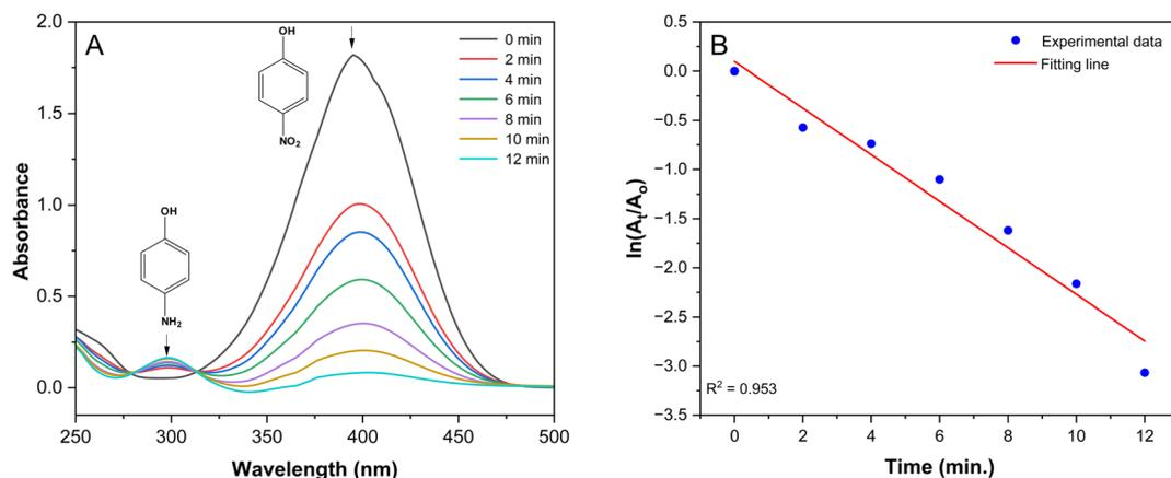
Fig. 8 UV-vis spectra of the reduction of 4-NP to 4-AP (A); pseudo-first-order reaction kinetics of the reduction of 4-NP to 4-AP (B). Reaction conditions: [4-NP] = 0.1 mM, [NaBH<sub>4</sub>] = 10 mM, 20 mg catalyst containing 8% of AgNPs.
