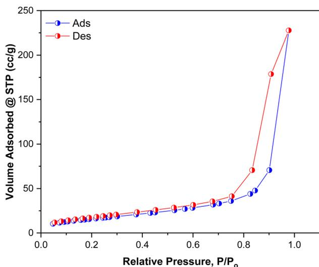
Fig. 7 N<sub>2</sub> adsorption-desorption isotherms of Ag/poly(AN-co-AMPS).
