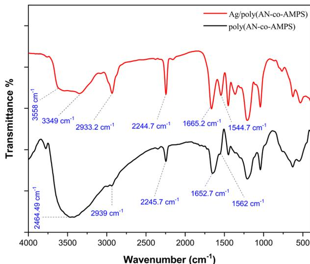
Fig. 2 FTIR spectra of poly(AN-co-AMPS) and Ag/poly(AN-co-AMPS).
