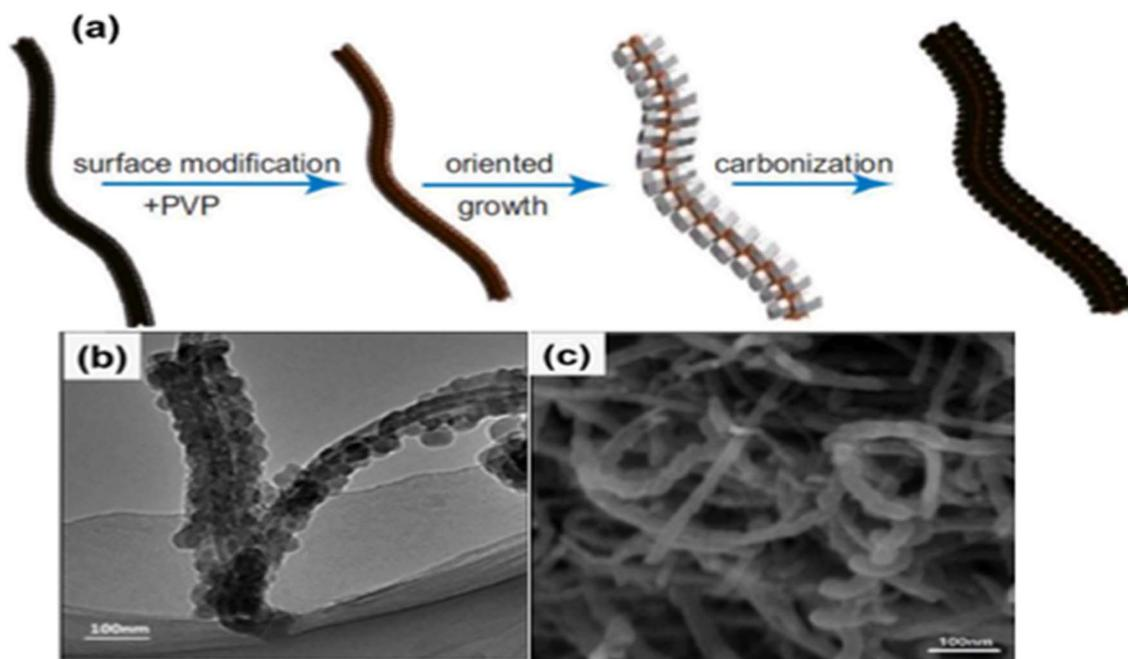
Fig. 9 (a) Synthesis method of ZIF-8@MWCNTs necklace-derived carbon, (b) and (c) the TEM and SEM images of the necklace-like ZIF-8@MWCNTs derived carbon.<sup>108</sup>
