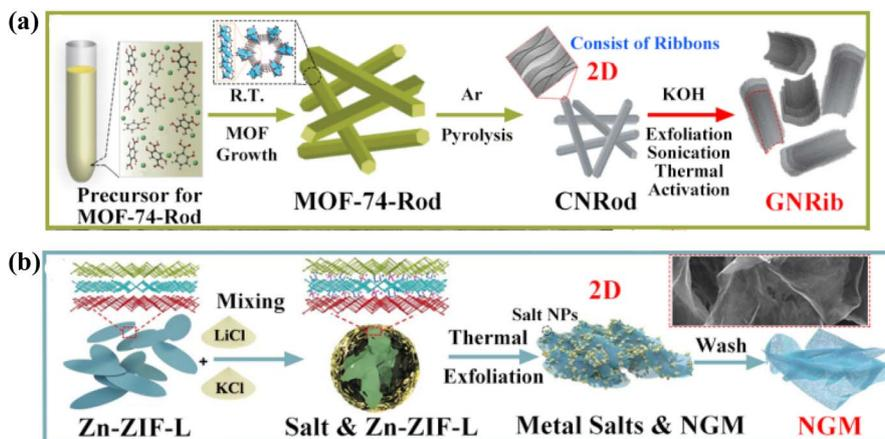
Fig. 11 (a) Preparation of MOF-derived 2D carbon nanorods and GNRRib.<sup>72</sup> (b) Preparation of MOF-derived 2D N-doped graphene nanomeses.<sup>125</sup>
