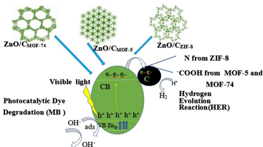
Fig. 16 The diagram illustrates the photocatalytic hydrogen evolution reaction (HER) activity of  $\text{ZnO/C}_{\text{MOF-5}}$ ,  $\text{ZnO/C}_{\text{MOF-74}}$ , and  $\text{ZnO/C}_{\text{ZIF-8}}$ , as well as their ability to degrade MB.
