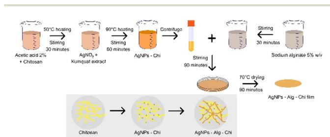
Fig. 1 The synthesis procedure for silver nanoparticles–sodium alginate–chitosan nanocomposite film. Alg: sodium alginate; AgNPs: silver nanoparticles; Chi: chitosan.
