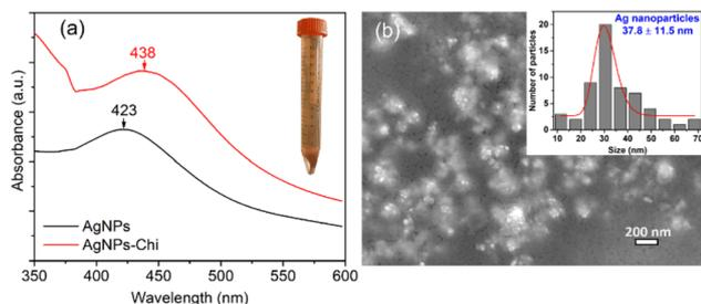
**Fig. 3** (a) UV-Vis absorption spectrum of an AgNPs and AgNPs-Chi ( $11 \mu\text{g mL}^{-1}$ ) prepared by mixing Kumquat extract with  $\text{AgNO}_3$ -Chitosan solution under heating at  $90^\circ\text{C}$  and magnetic stirring for 90 min; inset (a) is an Ag NPs-Chitosan solution. (b) SEM image of AgNPs solution, prepared by dropping the solution on Si substrate.
