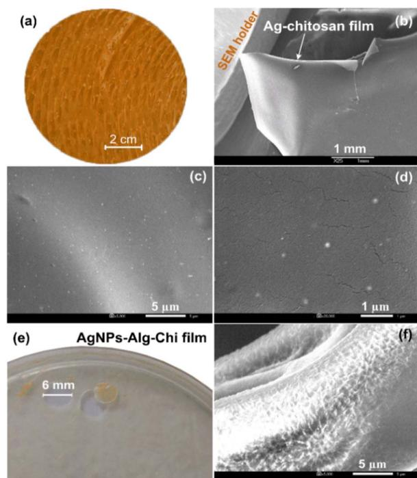
**Fig. 4** (a and b) A photograph and a low-magnification SEM of a typical Ag-Chi nanocomposite film. (c and d) SEM images of AgNPs-Chi solution prepared by dropping the solution onto a Si substrate. (e and f) Photograph and SEM image of AgNPs-Alg-Chi nanocomposite film.
