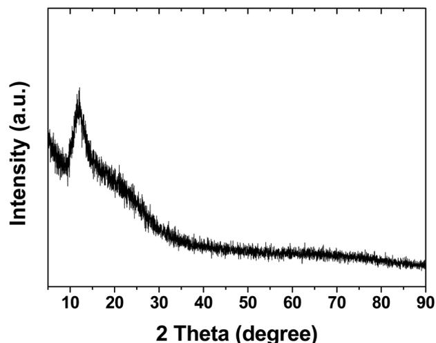
Fig. 5 X-ray diffraction pattern of PDMS powder.
