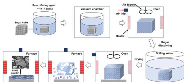
**Fig. 1** Schematic design of PDMS powder fabrication process.
