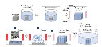
Fig. 1 Schematic design of PDMS powder fabrication process.
