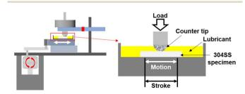
Fig. 2 Schematic diagram of the tribotester.
