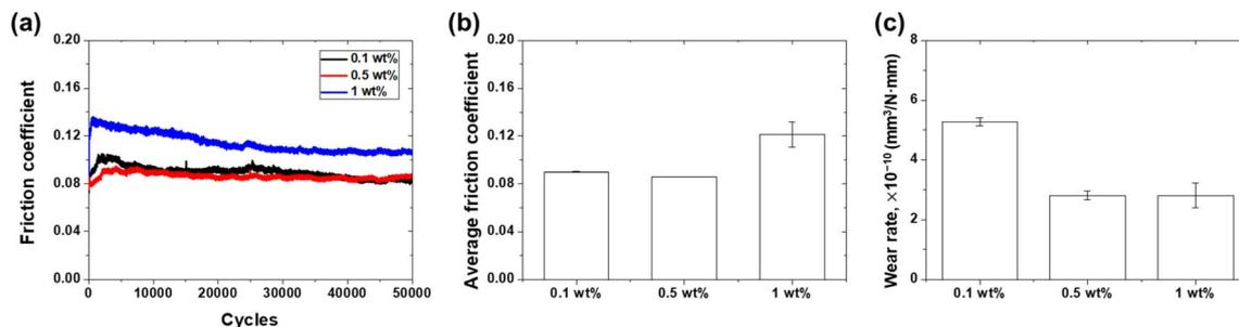
Fig. 11 Friction and wear characteristics of lubricants as a function of curing agent concentration: (a) friction coefficient history, (b) average friction coefficient, and (c) wear rate.
