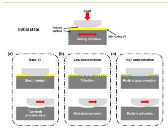
Fig. 13 Schematic design of the lubrication mechanism as a function of PDMS powder concentration: (a) 0 wt%, (b) 1-1.5 wt%, and (c) 2-2.5 wt%.
