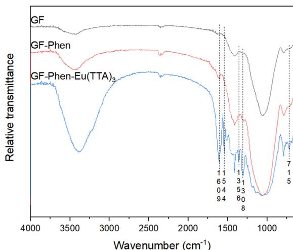
Fig. 1 FTIR spectra of GF, GF-Phen and GF-Phen-Eu(TTA)<sub>3</sub>.
