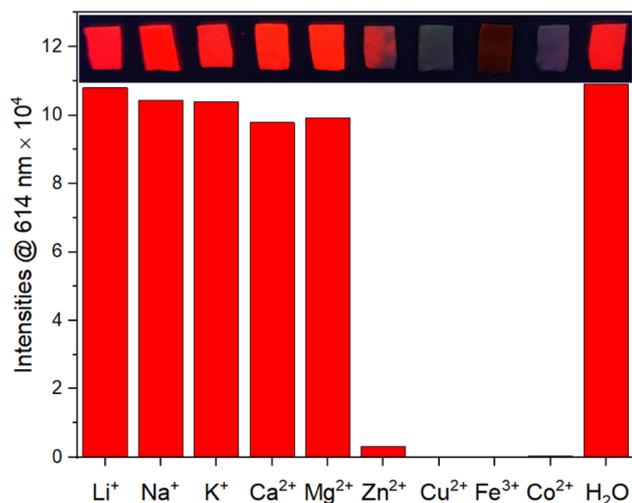
Fig. 4 Photographs of the GF-Phen-Eu(TTA)<sub>3</sub> strips under 365 nm UV lamp after treated with different metal ion solutions for 10 min, and comparison of their corresponding fluorescence intensity.
