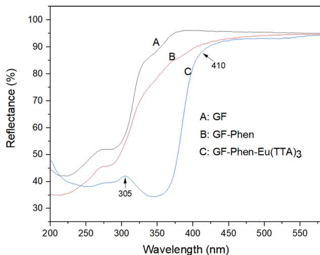
Fig. 2 UV-Vis DRS spectra of GF, GF-Phen and GF-Phen-Eu(TTA)<sub>3</sub>.
