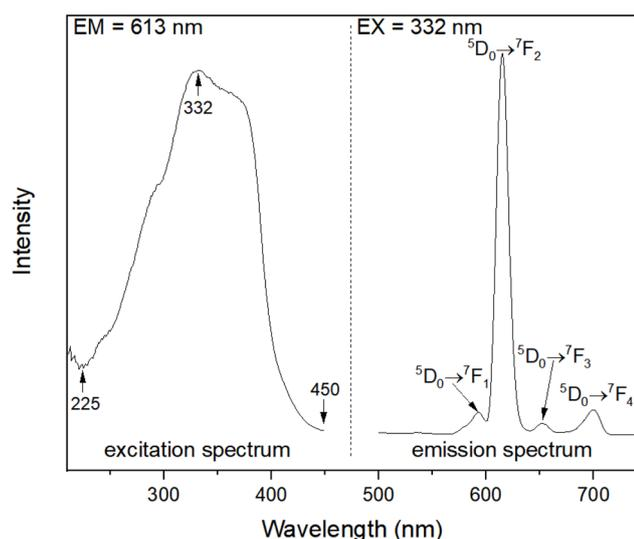
Fig. 3 Fluorescence excitation and emission spectra of GF-Phen-Eu(TTA)<sub>3</sub>.
