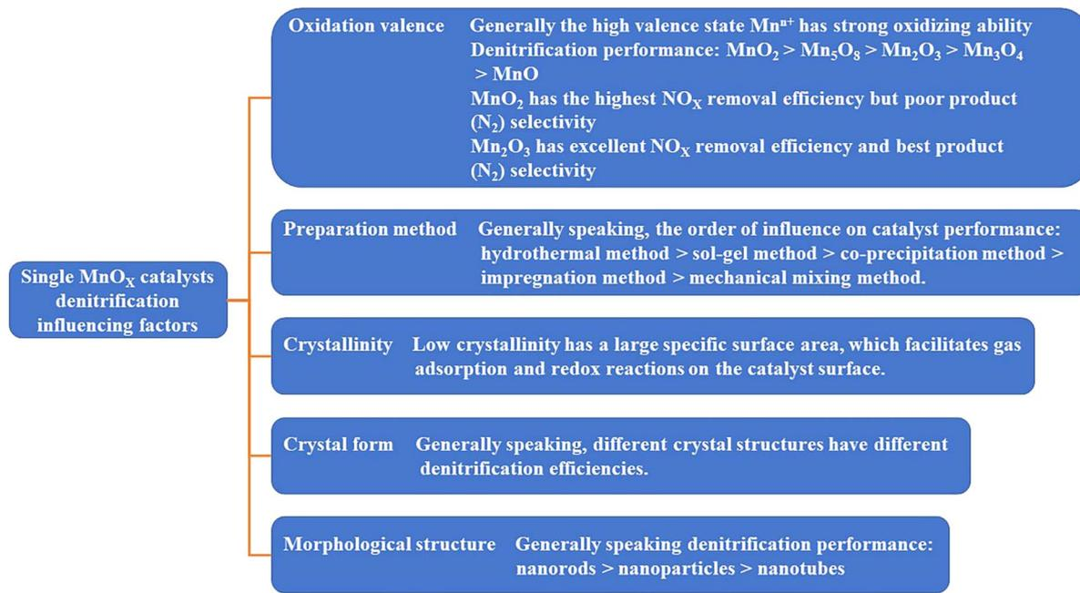
Fig. 4 Factors affecting the catalytic activity of single MnO<sub>x</sub> catalysts.
