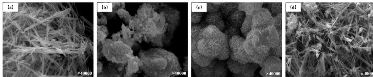
Fig. 2 The SEM images of four different  $\text{MnO}_2$  nanocrystals: (a)  $\alpha$ - $\text{MnO}_2$ ; (b)  $\beta$ - $\text{MnO}_2$ ; (c)  $\delta$ - $\text{MnO}_2$ ; (d)  $\gamma$ - $\text{MnO}_2$  (reprinted from ref. 32. Copyright 2017, with permission from Elsevier).
