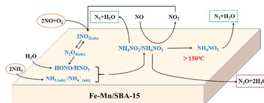
Fig. 13 Low temperature NH<sub>3</sub>-SCR reaction mechanism of Fe Mn/SBA-15 catalyst (reproduced from ref. 115 with permission from ACS Publications.).
