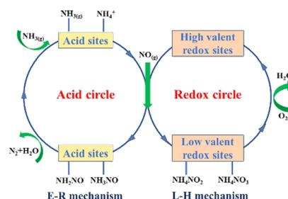
Fig. 9 Schematic diagram of NH<sub>3</sub>-SCR reaction pathway on metal oxide and zeolite catalysts (reproduced from ref. 29 with permission from ACS Publications).
