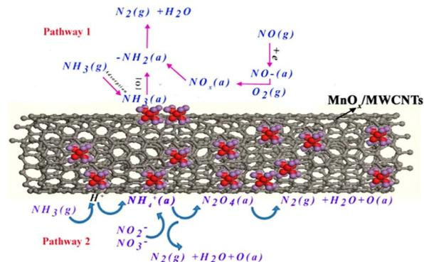
Fig. 15 Schematic diagram of two reaction pathways on MnO<sub>x</sub>/MWCNTs catalyst at 210 °C (reprinted from ref. 119. Copyright 2015, with permission from AAGR Aerosol and Air Quality Research).
