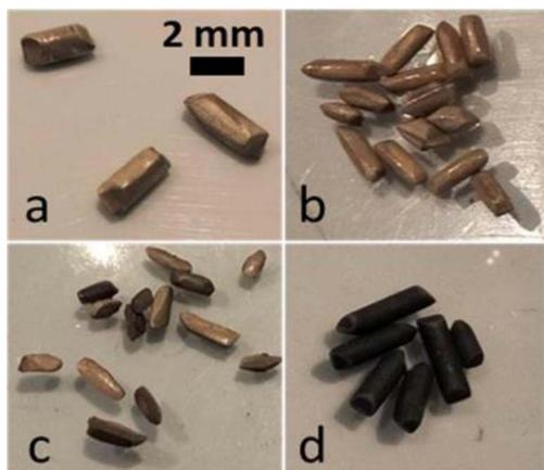
Fig. 5 Recovered Ag wires after 16 h of leaching with (a)  $0.03 \text{ mol L}^{-1}$ , (b)  $0.23 \text{ mol L}^{-1}$ , (c)  $0.40 \text{ mol L}^{-1}$  and (d)  $0.60 \text{ mol L}^{-1}$  of  $\text{FeCl}_3 \cdot 6\text{H}_2\text{O}$ .
