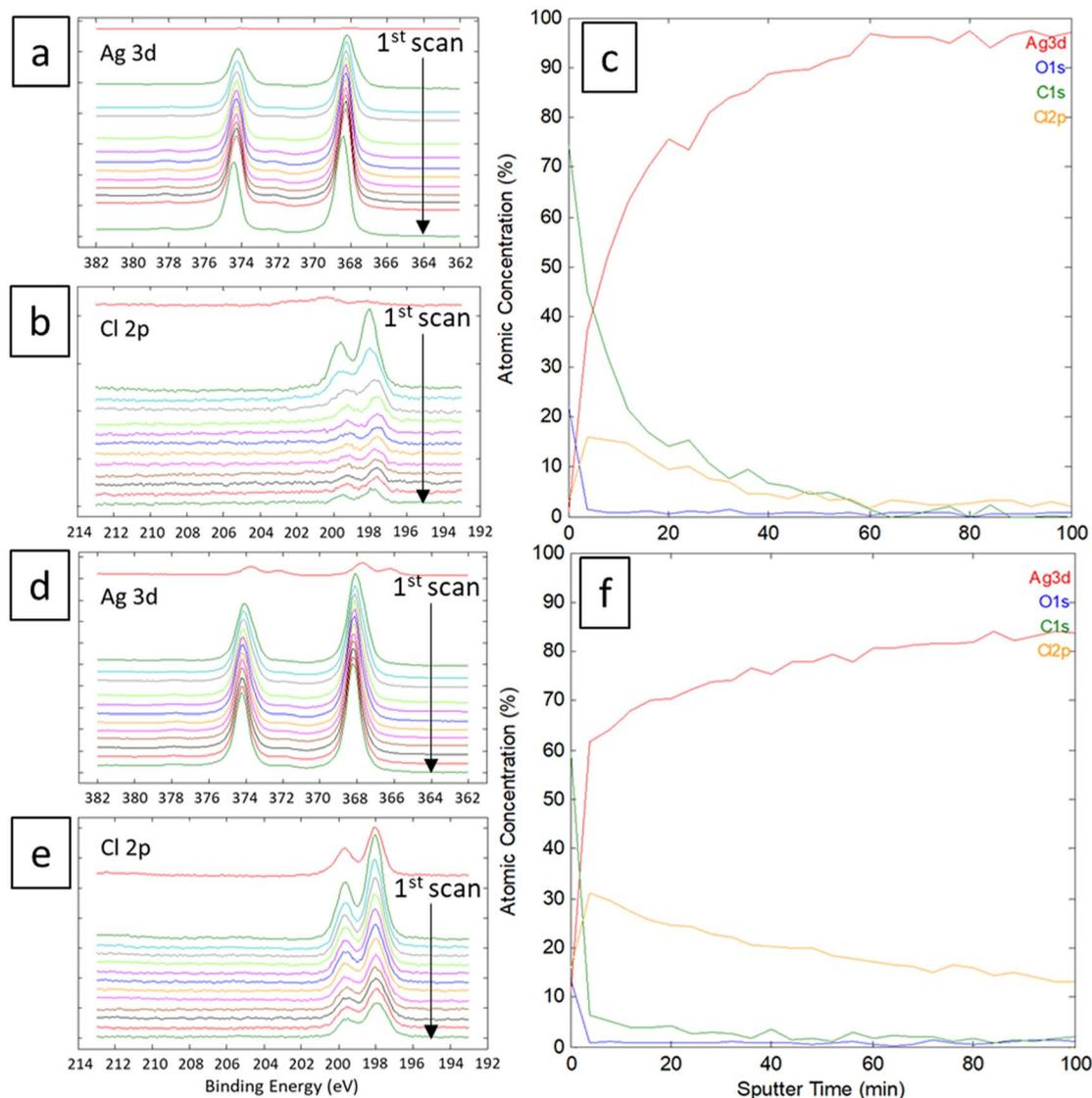
Fig. 6 XPS spectra focused on Ag and Cl of (a and b) Ag<sub>0.4</sub> and (d and e) Ag<sub>0.8</sub> wires during abrasion. Calculated atomic concentration in percentage of (c) Ag<sub>0.4</sub> and (f) Ag<sub>0.8</sub>.
