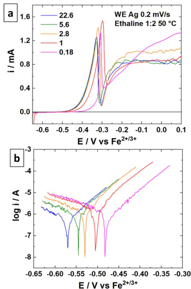
Fig. 4 (a) LSV curves of a Ag wire at 0.2 mV s<sup>-1</sup> and 50 °C in Ethaline 1:2 with different amounts of water. (b) Tafel plots of the LSV curves.
