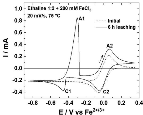
Fig. 3 Voltammograms of a Pt wire at 20 mV s<sup>-1</sup> and 75 °C in an Ethaline 1:2 + Fe<sup>3+</sup> 0.20 mol L<sup>-1</sup> solution before and after 6 h of leaching.
