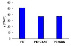
Fig. 3 Surface tension comparison between the extract containing CTAB and the extract containing SDS. Papaya extract (PE), papaya extract with CTAB (0.075 mM) (PE+CTAB), papaya extract with SDS (0.15 mM) (PE+SDS).
