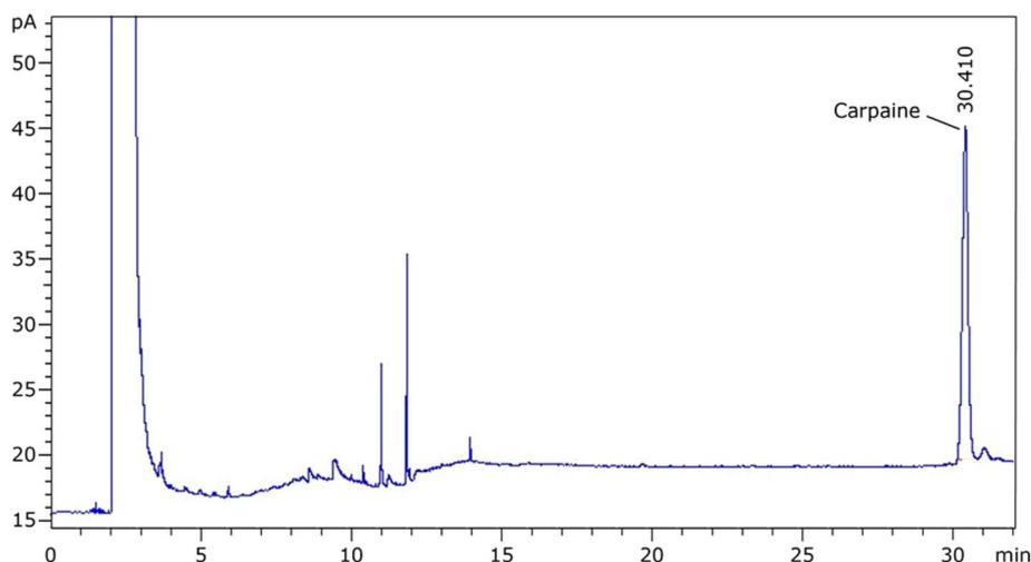
Fig. 9 GC-FID chromatogram of extracted carpaine after flotation.
