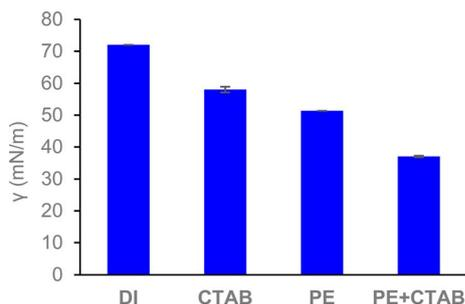
Fig. 2 Surface tension reduction due to saponin, CTAB and a combination of both; deionized water (DI), DI with CTAB (0.075 mM) (CTAB), papaya extract (PE), and papaya extract with CTAB (0.075 mM) (PE+CTAB).
