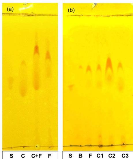
Fig. 4 Thin-layer chromatography analysis for carpaine visualization; (a) identification of carpaine; (b) comparison of carpaine in treatment sample with all controls, standard carpaine (S), carpaine–CTAB complex (C), carpaine–CTAB complex mixed with foam sample (C+F), control without flotation (B), foam sample (F), control without pre-incubation pH adjustment (C1), control without CTAB (C2), and control without pre-flotation pH adjustment (C3).
