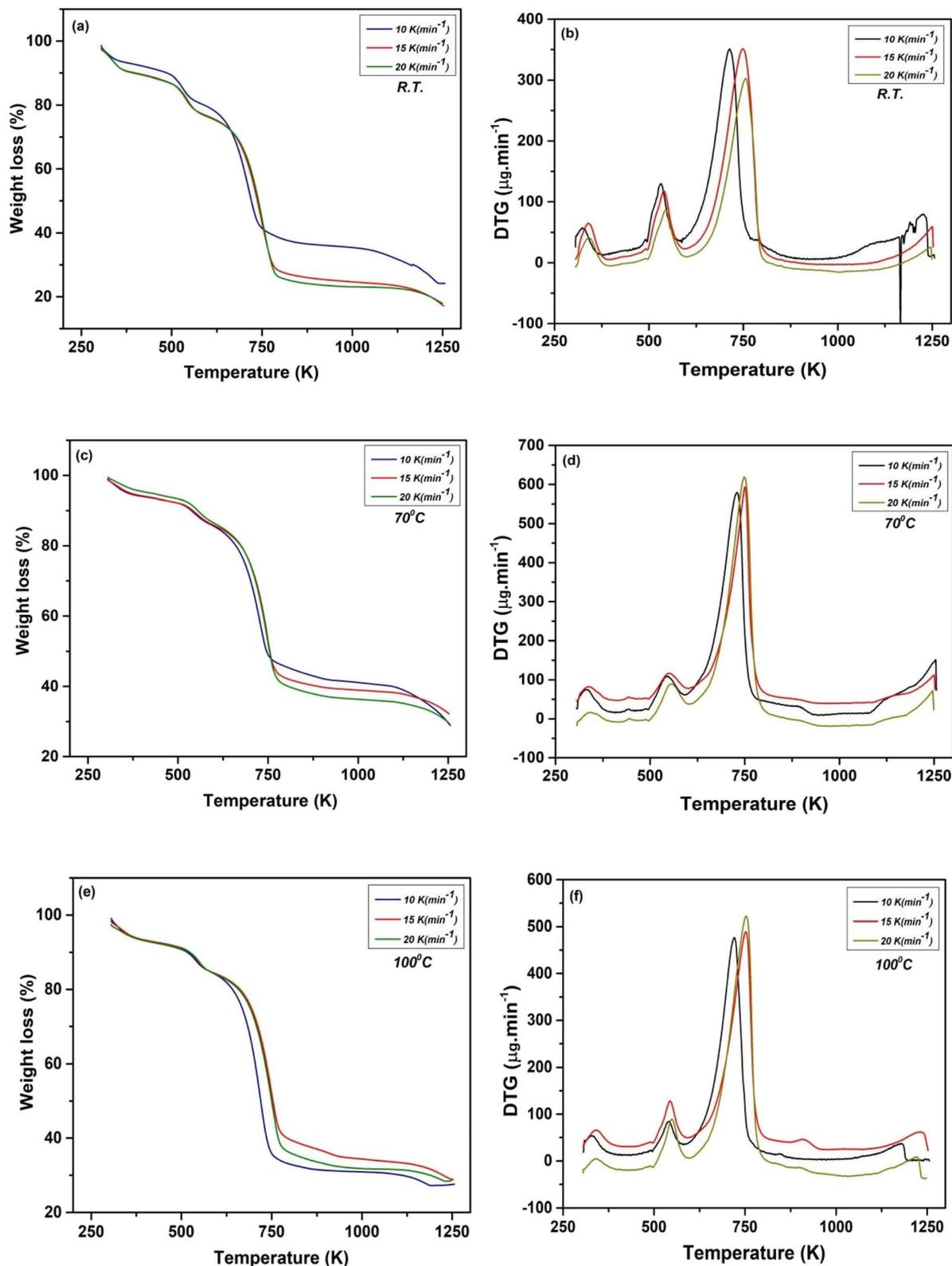
Fig. 4 TG curves of NbSe<sub>2</sub> NPs synthesized at (a) R.T., (c) 70 °C, (e) 100 °C and DTG curve of NbSe<sub>2</sub> NPs synthesized at (b) R.T., (d) 70 °C and (f) 100 °C.
