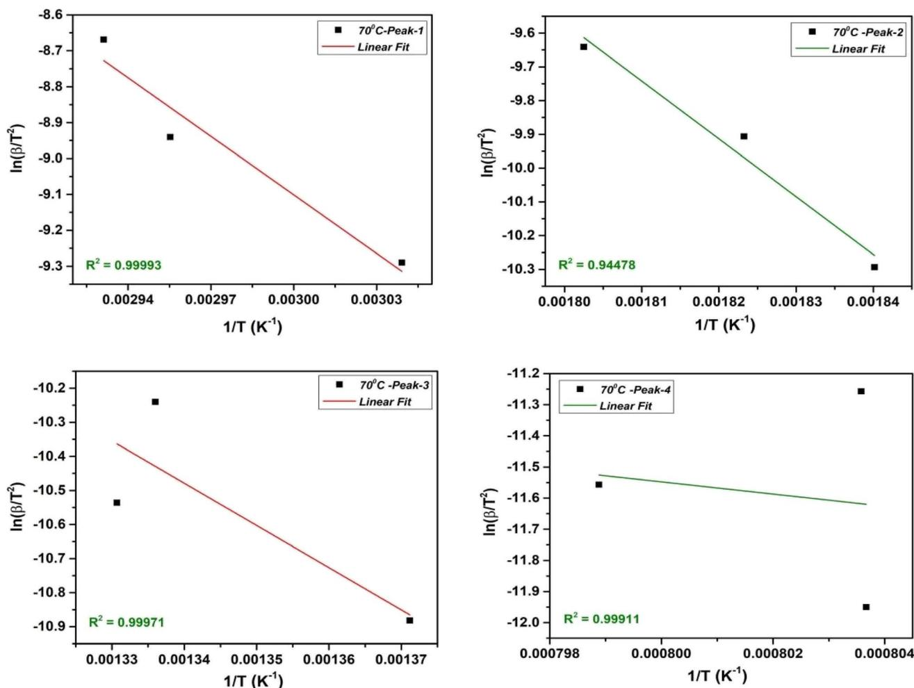
Fig. 6 The KAS plot of four step decomposition for NbSe<sub>2</sub> NPs sample synthesized at 70 °C.
