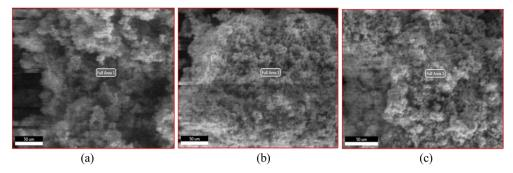
Fig. 2 Shows the microscopic image from EDAX for NbSe<sub>2</sub> nanoparticles synthesized at (a) R.T., (b) 70 °C, (c) 100 °C respectively.
