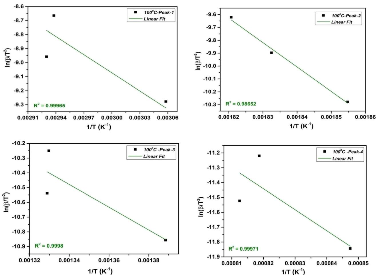
Fig. 7 The KAS plot of four-step decomposition for NbSe<sub>2</sub> NPs sample synthesized at 100 °C.
