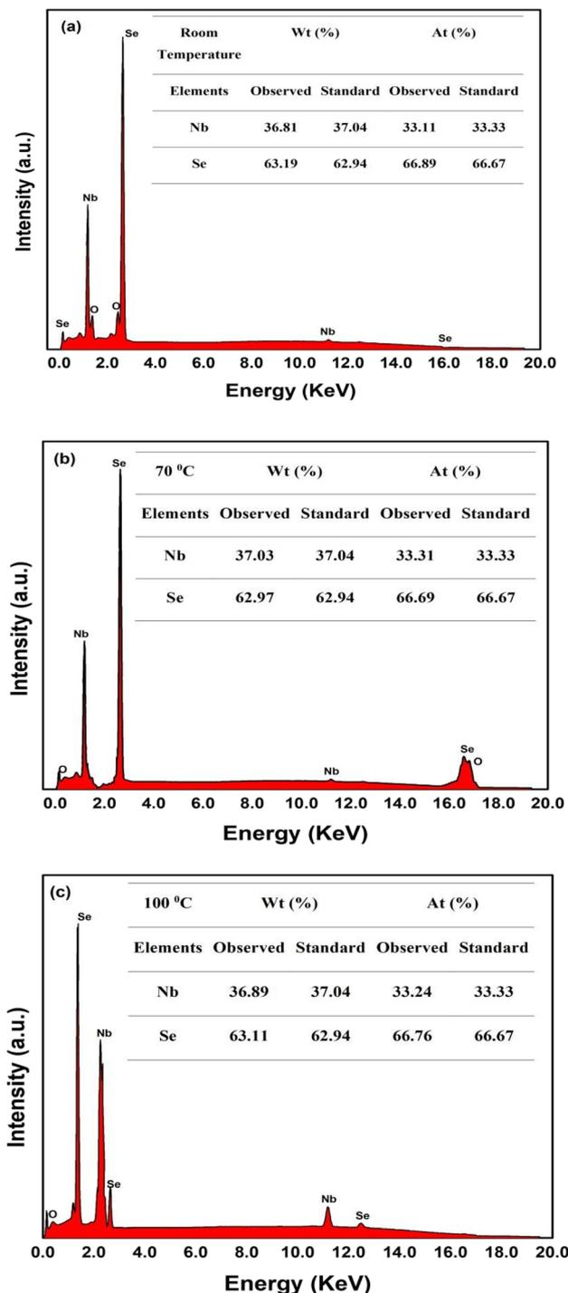
Fig. 1 The EDAX spectrum of NbSe<sub>2</sub> NPs synthesized at (a) R.T., (b) 70 °C, and (c) 100 °C.
