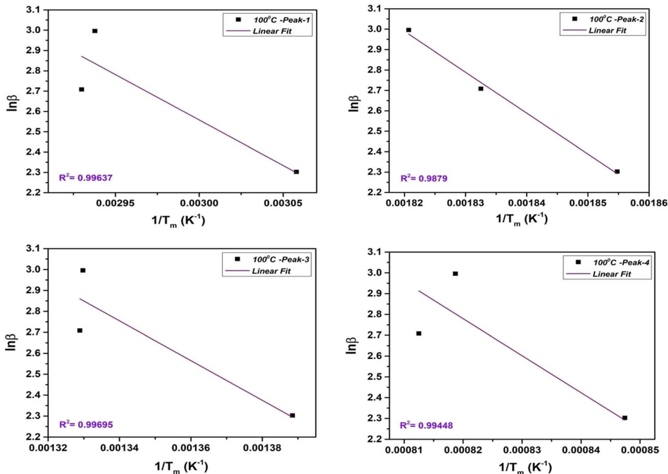
Fig. 10 The FWO plot of four-step decomposition for NbSe<sub>2</sub> NPs sample synthesized at 100 °C.
