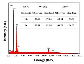
Fig. 1 The EDAX spectrum of NbSe $_2$  NPs synthesized at (a) R.T., (b) 70  $^\circ$  C, and (c) 100  $^\circ$ C.
