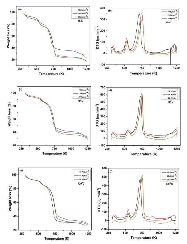
Fig. 4 TG curves of NbSe<sub>2</sub> NPs synthesized at (a) R.T., (c) 70 °C, (e) 100 °C and DTG curve of NbSe<sub>2</sub> NPs synthesized at (b) R.T., (d) 70 °C and (f) 100 °C.
