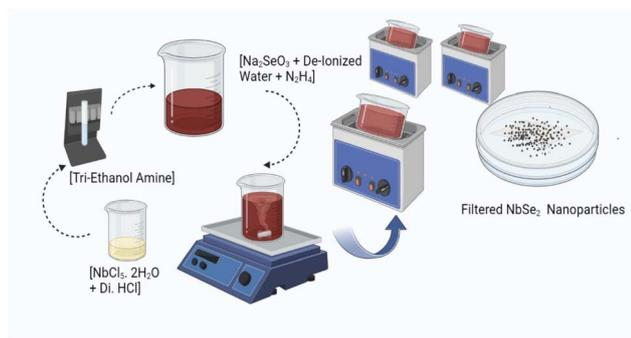
Fig. 11 Shows the schematic illustration of the synthesis of NbSe<sub>2</sub> nanoparticles synthesized at R.T., 70 °C, and 100 °C via the sonochemical method.
