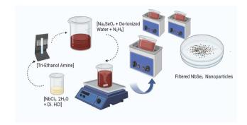
Fig. 11 Shows the schematic illustration of the synthesis of NbSe $_2$  nanoparticles synthesized at R.T., 70 °C, and 100 °C  $\it via$  the sonochemical method.
