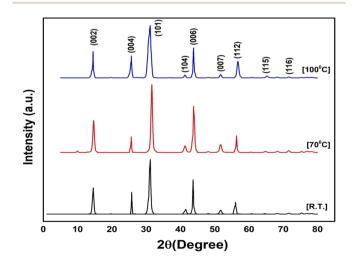
Fig. 3 The XRD patterns of NbSe<sub>2</sub> NPs samples synthesized at R.T., 70 °C, and 100 °C.
