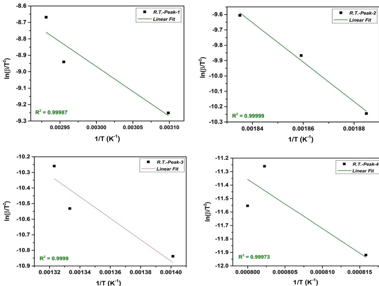
Fig. 5 The KAS plot of four-step decomposition for NbSe<sub>2</sub> NPs sample synthesized at R.T.
