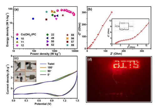
Fig. 7 (a) Ragone plot of the solid-state  $Co(OH)_2/PC$  ASC device with a comparison of reported research on  $Co(OH)_2$ -based supercapacitors, (b) Nyquist plot, and (c) CV test with different angles of the solid-state ASC device. (d) LED light illuminated by the solid-state ASC device.
