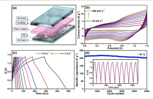
Fig. 6 (a) Graphical sketch of a solid-state Co(OH)<sub>2</sub>//PC ASC device. (b) CV scans and (c) GCD curves of the solid-state Co(OH)<sub>2</sub>//PC ASC device. (d) Cycling stability test (inset: first GCD 10 cycles) of the device.
