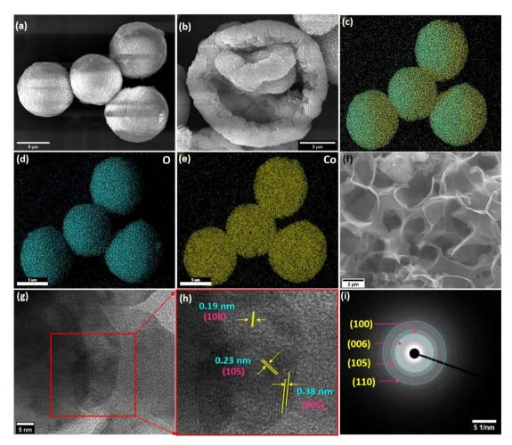
Fig. 2 (a and b) FESEM images of Co(OH)<sub>2</sub>. EDS elemental color mapping of Co(OH)<sub>2</sub>: (c) overlay, (d) O, and (e) Co. (f) FESEM image of porous carbon. (g and h) HRTEM images and (i) SAED pattern of Co(OH)<sub>2</sub>.
