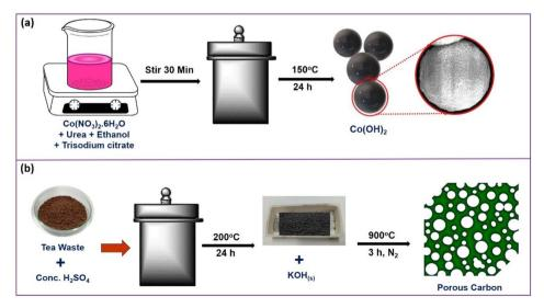
Scheme 1 Graphical illustration of the synthesis routes for (a) Co(OH)<sub>2</sub> and (b) porous carbon.
