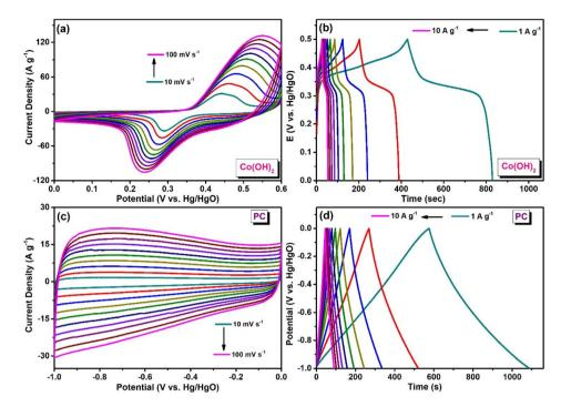
Fig. 4 (a) CV curves and (b) GCD curves of Co(OH)<sub>2</sub>. (c) CV curves and (d) GCD curves of PC in 3 M KOH.
