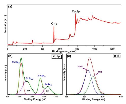
Fig. 3 XPS spectra of Co(OH)<sub>2</sub>: (a) survey spectrum, (b) Co 2p, and (c) O 1s.
