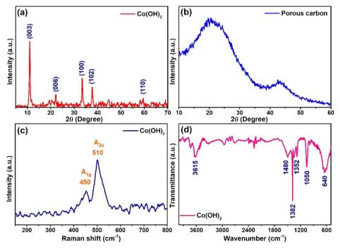
Fig. 1 XRD pattern of (a) Co(OH)<sub>2</sub> and (b) porous carbon. (c) Raman spectra and (d) FTIR spectra of Co(OH)<sub>2</sub>
