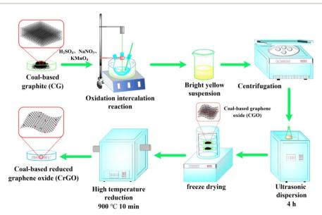
Fig. 1 Preparation flow chart of CrGO.
