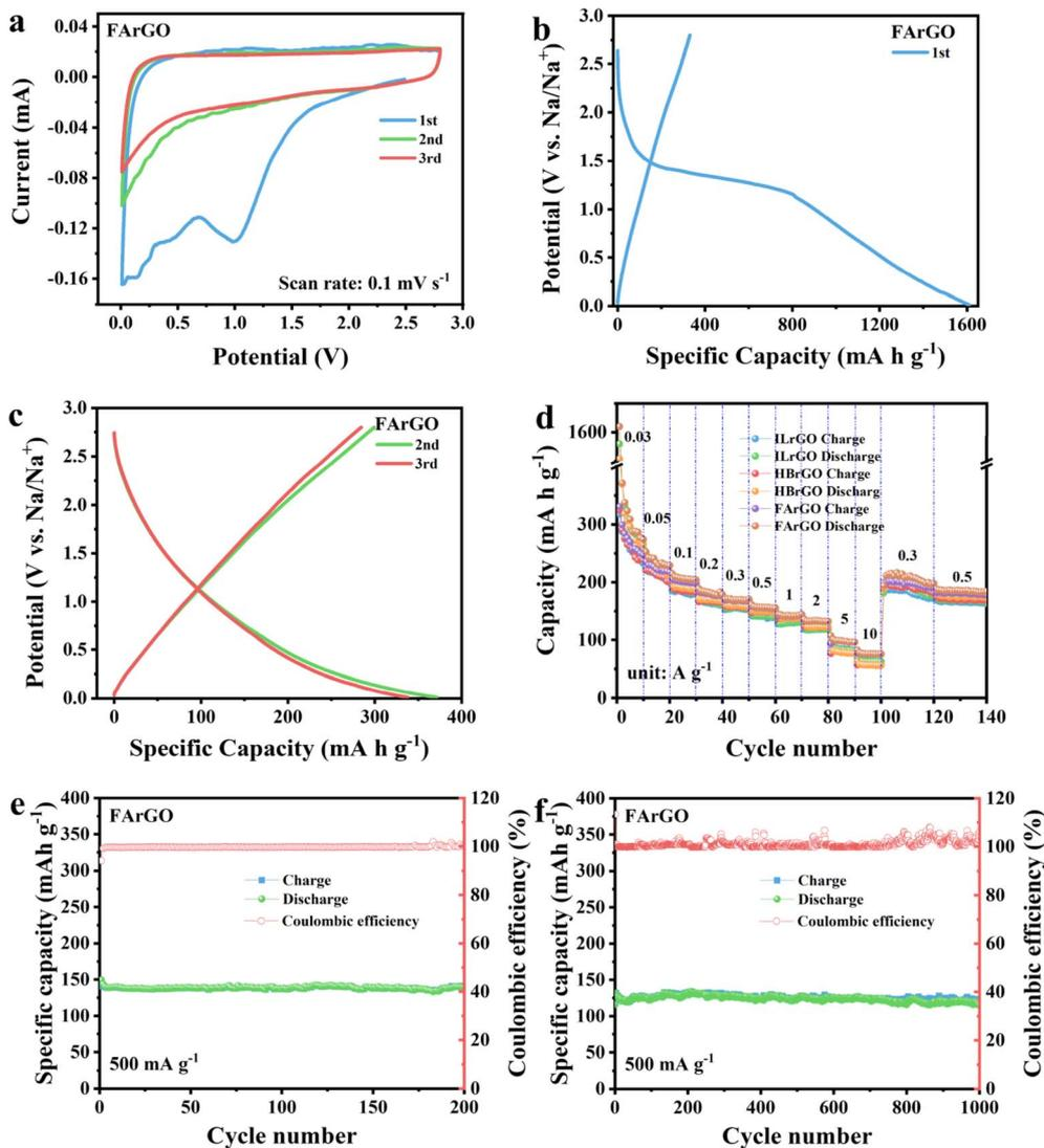
Fig. 4 The first three CV curves of FArGO (a), first three charge/discharge curves of FArGO (b and c), rate performance (d) of ILrGO, HBrGO, and FArGO, cycling stability of FArGO at 0.5 and 1 A g<sup>-1</sup>.
