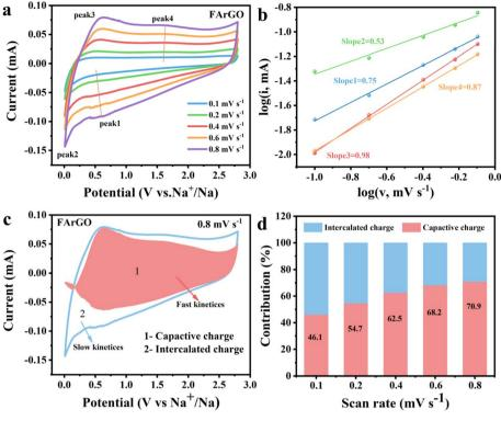
Fig. 5 The CV curves at different scan rate range between 0.1 and 0.8 mV s<sup>-1</sup> of FArGO (a). The relationship between logarithm of peak current and logarithm of scan rates (b). The capacitive contribution in CV curves of FArGO at 0.8 mV s<sup>-1</sup> (c). The capacitance contribution of FArGO at different scan rates (d).
