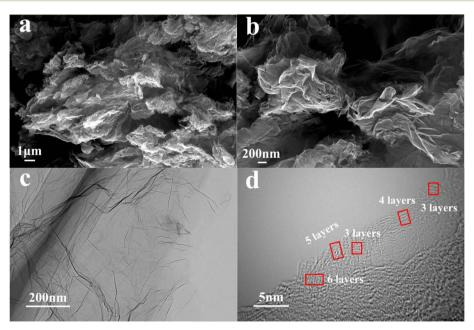
Fig. 2 SEM images (a and b), TEM images (c) and HRTEM images (d) of FArGO.
