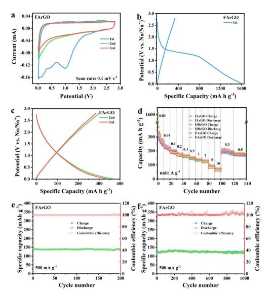
Fig. 4 The first three CV curves of FArGO (a), first three charge/discharge curves of FArGO (b and c), rate performance (d) of ILrGO, HBrGO, and FArGO, cycling stability of FArGO at 0.5 and 1 A  $g^{-1}$ .
