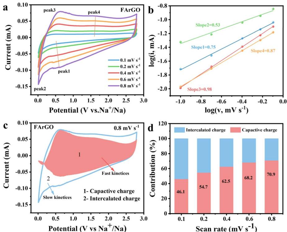
Fig. 5 The CV curves at different scan rate range between 0.1 and 0.8  $\text{mV s}^{-1}$  of FarGO (a). The relationship between logarithm of peak current and logarithm of scan rates (b). The capacitive contribution in CV curves of FarGO at 0.8  $\text{mV s}^{-1}$  (c). The capacitance contribution of FarGO at different scan rates (d).
