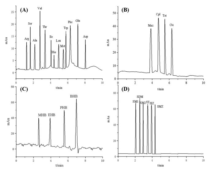
Fig. 10 Separation chromatogram of 13 amino acids (A), 4 antibiotics (B), 4 preservatives (C) and 6 sulfonamides (D) on the TpBD/UiO-66-NH<sub>2</sub>-bonded OT-CEC column under optimized CEC conditions (experimental conditions: 20 mmol  $L^{-1}$  of ammonium acetate buffer; pH = 8 for amino acids, pH = 9 for the other analytes; operating voltage, 15 kV; detection wavelength, amino acids at 214 nm, sulfonamides at 254 nm, and others at 270 nm.).
