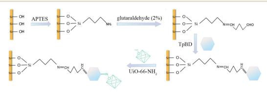
Fig. 2 Preparation scheme for the TpBD/UiO-66-NH<sub>2</sub>-bonded OT-CEC column.
