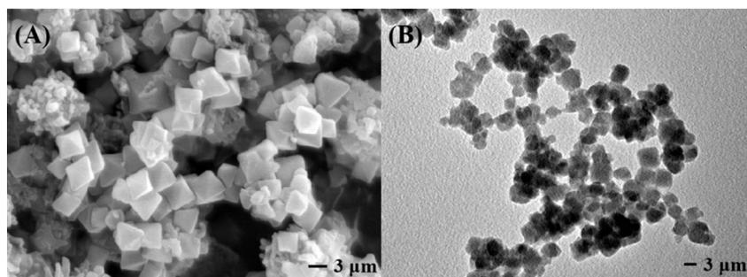
Fig. 5 SEM (A) and TEM (B) images of TpBD/UiO-66-NH<sub>2</sub>.
