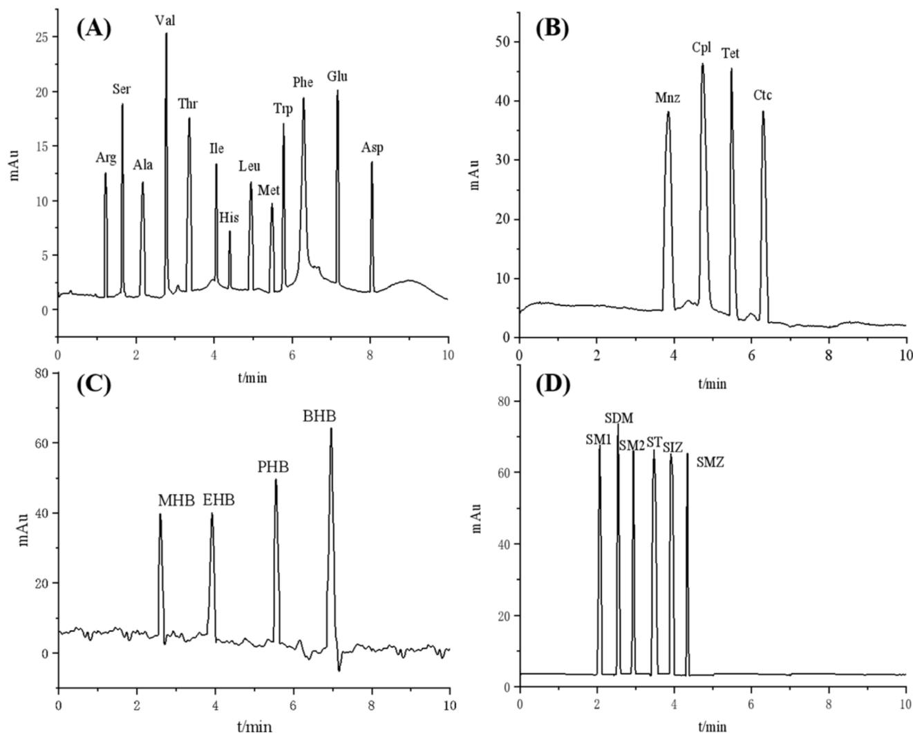
Fig. 10 Separation chromatogram of 13 amino acids (A), 4 antibiotics (B), 4 preservatives (C) and 6 sulfonamides (D) on the TpBD/Uio-66-NH<sub>2</sub>-bonded OT-CEC column under optimized CEC conditions (experimental conditions: 20 mmol L<sup>-1</sup> of ammonium acetate buffer; pH = 8 for amino acids, pH = 9 for the other analytes; operating voltage, 15 kV; detection wavelength, amino acids at 214 nm, sulfonamides at 254 nm, and others at 270 nm.).
