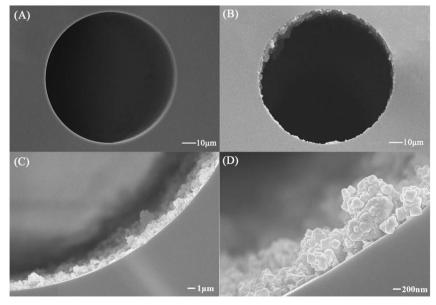
Fig. 9 SEM images of the cross section of the bare capillary column (A) and the TpBD/UiO-66-NH<sub>2</sub>-bonded OT-CEC column (B-D).
