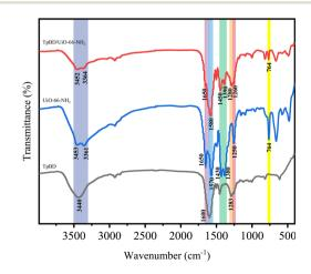
Fig. 4 FT-IR spectra of TpBD, UiO-66-NH<sub>2</sub>, and TpBD/UiO-66-NH<sub>2</sub>.
