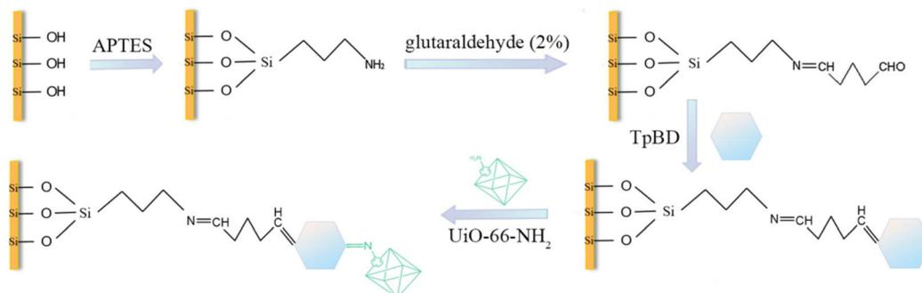
Fig. 2 Preparation scheme for the TpBD/UiO-66-NH<sub>2</sub>-bonded OT-CEC column.
