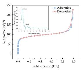
Fig. 7  $N_2$  adsorption–desorption isotherms of TpBD/UiO-66-NH<sub>2</sub> at 77.3 K ((inset): pore size distribution).
