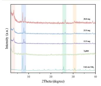
Fig. 3 XRD spectra of TpBD/UiO-66-NH<sub>2</sub> (experimental conditions: TpBD dosage, 27.8 mg; reaction temperature, 80 °C; reaction time, 24 h), TpBD and UiO-66-NH<sub>2</sub>.
