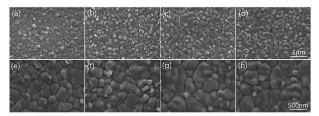
Fig. 4 Surface SEM images of  $CH_3NH_3Pbl_3$  thin films treated with different concentrations of AA at EA values of 0 (a and e), 0.5% (b and f), 1% (c and g), and 2% (d and h). This figure has been reproduced from ref. 39 with permission from Elsevier, copyright 2022.
