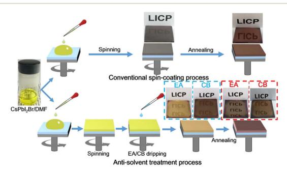
Fig. 2 Schematic diagram of traditional spin coating and anti-solvent treatment processes for manufacturing perovskite thin films (using EA and CB). This figure has been reproduced from ref. 36 with permission from Wiley, copyright 2018
