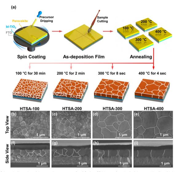
Fig. 9 (a) Schematic illustration of the annealing processes. (b–e) Surface SEM images (top view) of the perovskite films fabricated through HTSA-100, HTSA-200, HTSA-300, and HTSA-400 and (f–i) their cross-sectional images (side view), respectively. This figure has been reproduced from ref. 85 with permission from American Chemical Society, copyright 2017.
