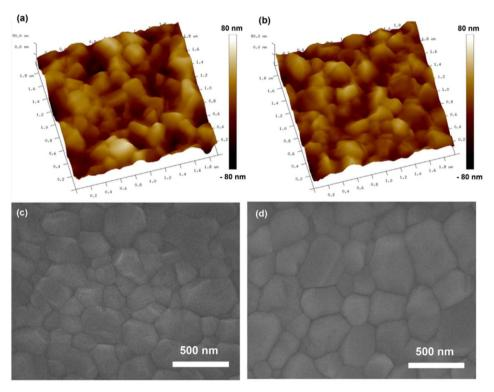
Fig. 6 Microstructure of perovskite thin films deposited on  $TiO_2/FTO$  substrates: AFM morphology images of (a) CB-P, (b) PhOMe-P, and corresponding surface SEM images of (c) CB-P, (d) PhOMe-P. This figure has been reproduced from ref. 49 with permission from Wiley, copyright 2018.
