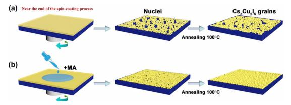
Fig. 8 Growth and grain growth of Cs<sub>3</sub>Cu<sub>2</sub>I<sub>5</sub> perovskite film with/without MA, (a) without MA. (b) With MA. This figure has been reproduced from ref. 58 with permission from Elsevier, copyright 2020
