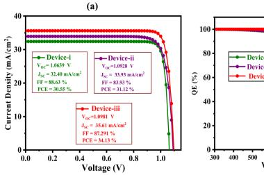
Fig. 14 (a) J-V and (b) Q-E curves of Device-I. II, and III structures.
