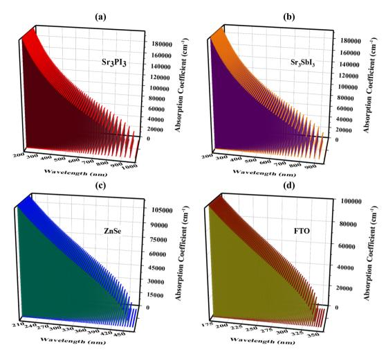
Fig. 4 Absorption coefficient of Al/FTO/ZnSe/absorber (Sr<sub>3</sub>Sbl<sub>3</sub>//Sr<sub>3</sub>Sbl<sub>3</sub>)/Au ideal solar cell construction for the following materials: (a) Sr<sub>3</sub>Pl<sub>3</sub>, (b) Sr<sub>3</sub>Sbl<sub>3</sub>, (c) ZnSe, and (d) FTO.
