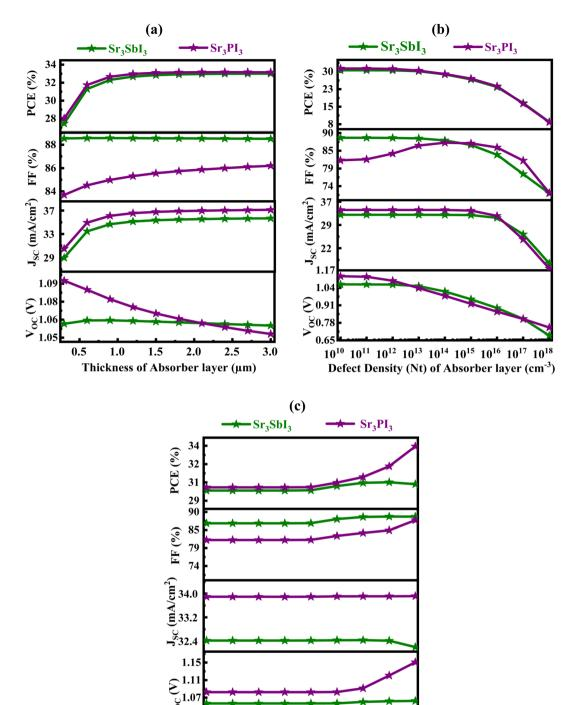
Fig. 5 Impact of (a) thickness, (b) defect density, and (c) doping concentration of absorber layer on the solar cell's performance for Devices I and II.
