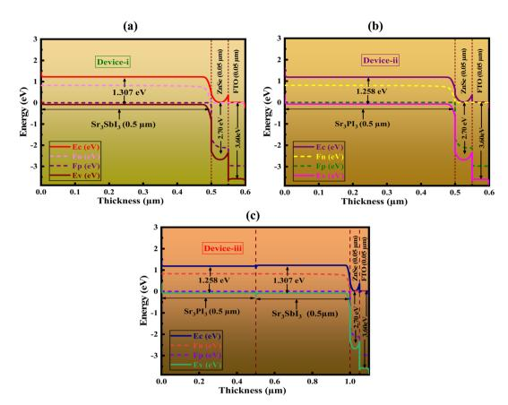
Fig. 3 Band arrangement of three types of HTL-free PSCs, featuring different light absorber materials: (a) Sr<sub>3</sub>Sbl<sub>3</sub>, (b) Sr<sub>3</sub>Pl<sub>3</sub>, (c) Sr<sub>3</sub>Pl<sub>3</sub>/Sr<sub>3</sub>Sbl<sub>3</sub> bilayer combination.
