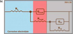
Scheme 3 Electrical equivalent circuit (a) uncoated 316 L SS and etched 316 L SS, (b) PAN coated 316 L SS and PAN-CMQD coated 316 L SS
