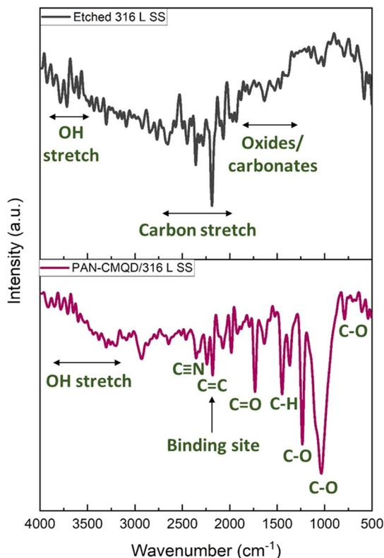
Fig. 2 FTIR spectra of etched and PAN-CMQD/316 L SS.
