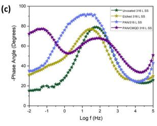
Fig. 8 (a) Nyquist plot for uncoated 316 L SS, etched 316 L SS, PAN coated 316 L SS and PAN-CMQD coated 316 L SS. (b) Bode plot for uncoated 316 L SS, etched 316 L SS, PAN coated 316 L SS and PAN-CMQD coated 316 L SS. (c) Phase angle plot for uncoated 316 L SS, etched 316 L SS, PAN coated 316 L SS and PAN-CMQD coated 316 L SS.
