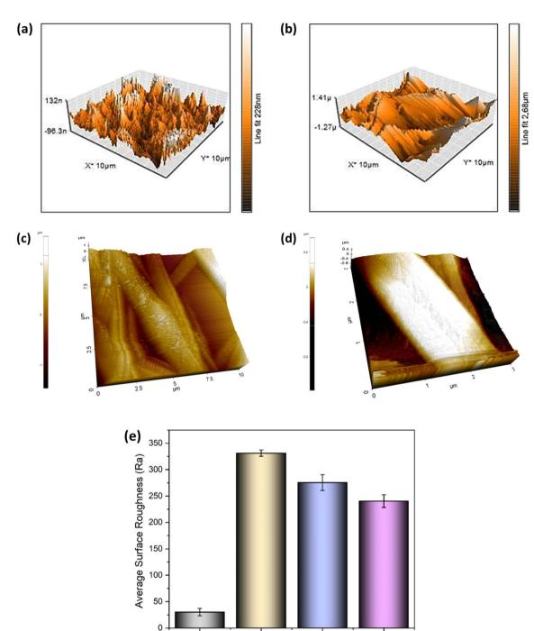
Fig. 4 AFM images of (a) uncoated, (b) etched, (c) PAN/316 L SS (d) PAN-CMQD/316 L SS. (e) Surface roughness of uncoated, etched, PAN/316 L SS and PAN-CMQD/316 L SS.
