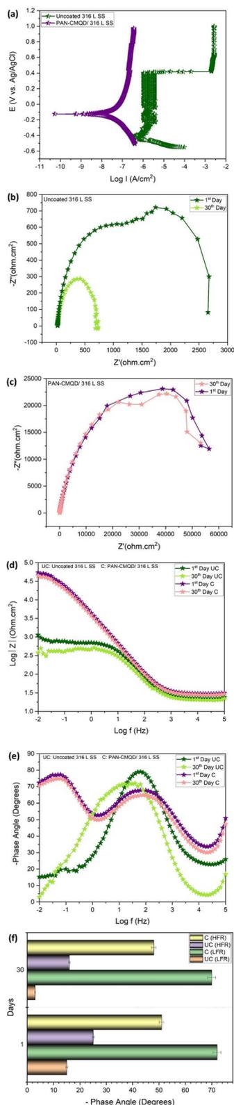
**Fig. 9** Long term corrosion resistance (a) PD plot of uncoated and PAN-CMQD coated 316 L SS after 30 days exposure in corrosive environment. (b) Nyquist plot of uncoated 316 L SS on 1st day and 30th day exposure in corrosive environment. (c) Nyquist plot of PAN-CMQD coated 316 L SS on 1st day and 30th day exposure in corrosive environment. (d) Bode plot of uncoated and PAN-CMQD coated 316 L SS on 1st day and 30th day exposure in corrosive environment. (e) Phase
