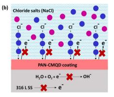
Scheme 4 Corrosion inhibition mechanism (a) uncoated 316 L SS (b) PAN-CMQD coated 316 L SS.
