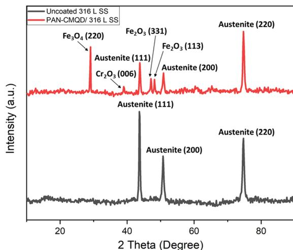
Fig. 6 XRD of uncoated and PAN-CMQD/316 L SS.
