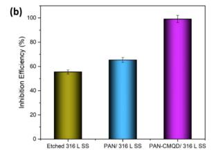
Fig. 7 (a) PD plot (b) inhibition efficiency (IE) from Tafel plot.
