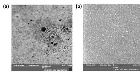
Fig. 10 SEM micrographs of 316 L SS (a) uncoated sample after 30 days exposure to corrosive environment (b) PAN-CMQD coated etched sample after 30 days exposure to corrosive environment.
