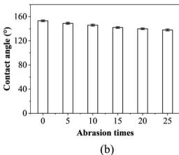
Fig. 8 CA variations of the replica surfaces after (a) the adhesive tape peeling test and (b) sandpaper abrasion.
