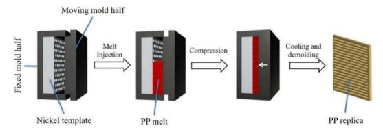
Fig. 1 Illustration of preparation process of the PP replica by the ICM technique.
