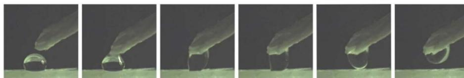
Fig. 6 Snapshots of the water droplet transfer test on the PP replica surface.
