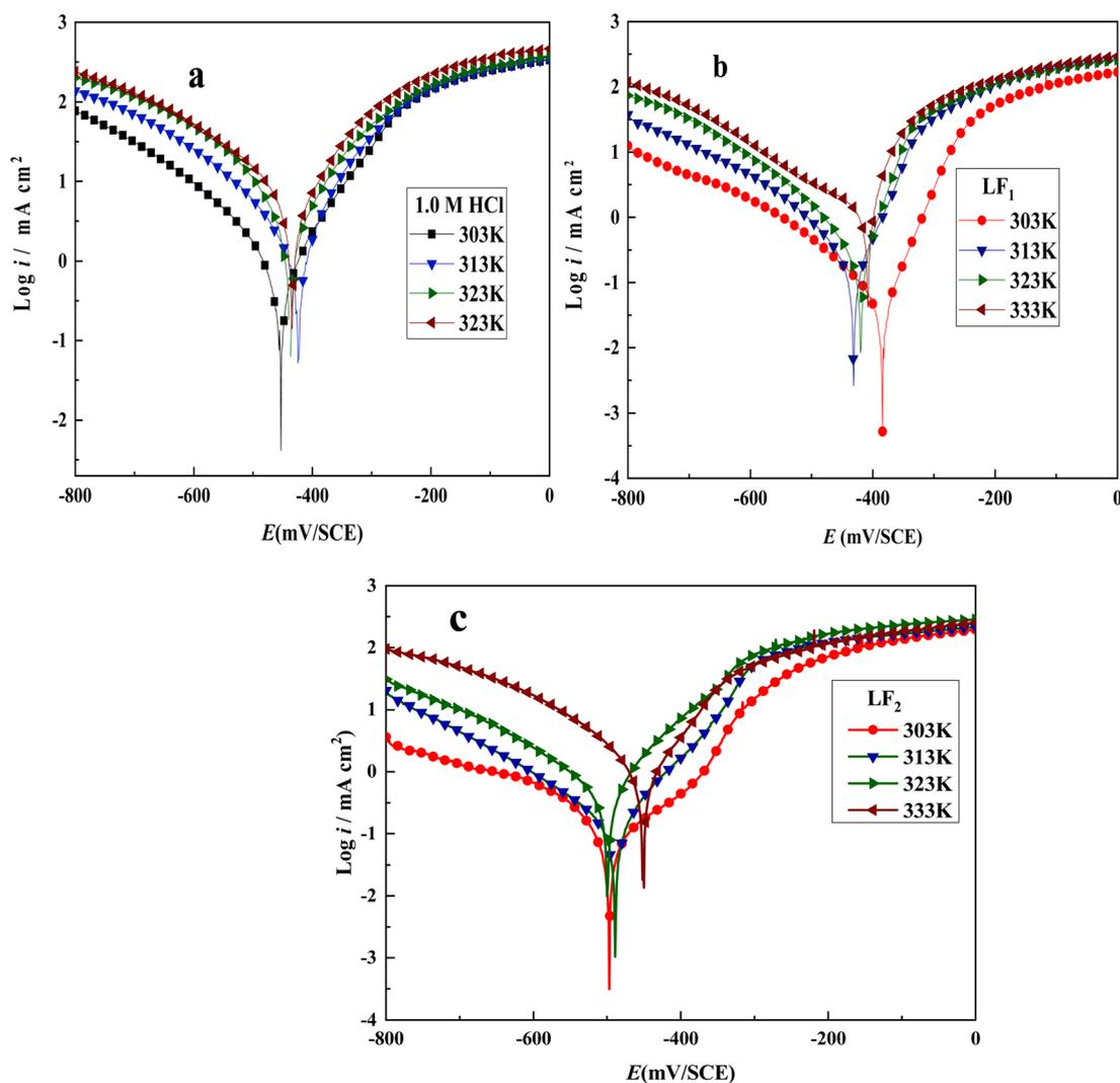
Fig. 4 Tafel plots showing C.S in 1.0 M HCl solution with and without inhibitors at  $10^{-3}$  M concentrations at varying temperatures: (a) without inhibitor, (b) with LF<sub>1</sub>, and (c) with LF<sub>2</sub>.
