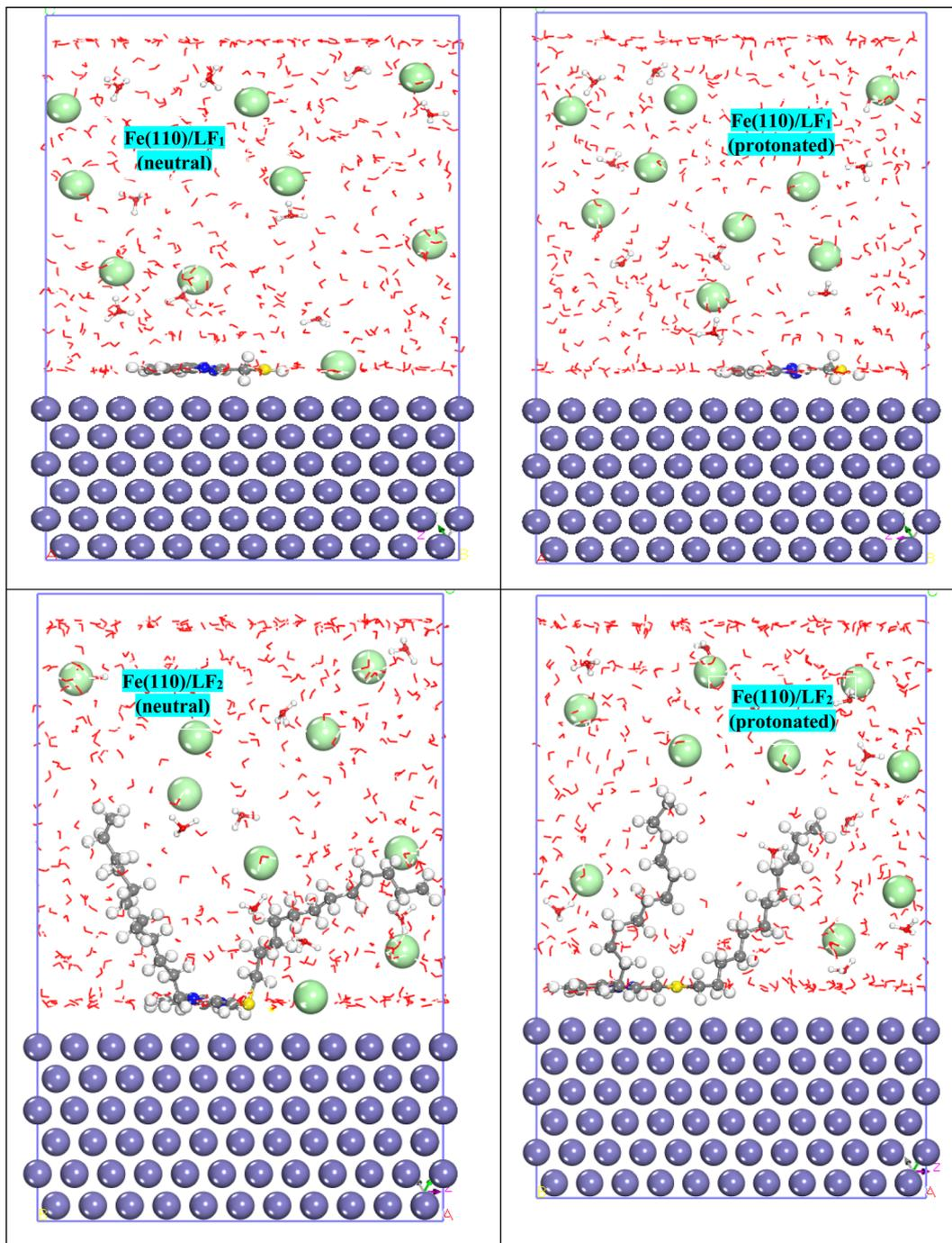
Fig. 12 Adsorption configurations feature the most stable forms for the systems Fe(110)/LF<sub>1</sub> (neutral), Fe(110)/LF<sub>2</sub> (neutral), Fe(110)/LF<sub>1</sub> (protonated), and Fe(110)/LF<sub>2</sub> (protonated).
