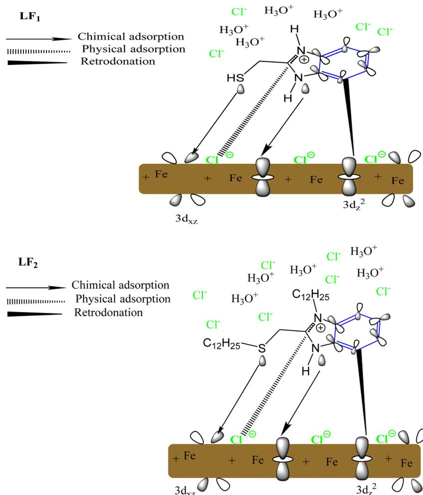
Fig. 14 Proposed mechanism of corrosion inhibition of LF<sub>1</sub> and LF<sub>2</sub>.
