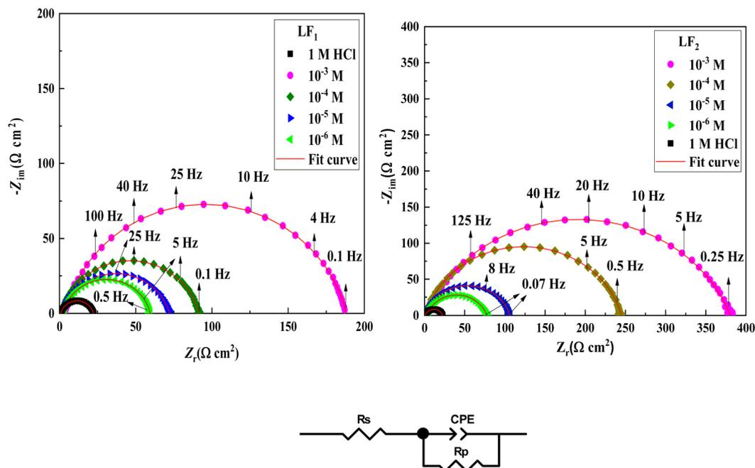
Fig. 2 Impedance spectroscopy Nyquist plots in a 1.0 M HCl solution at various  $LF_1$  and  $LF_2$  concentrations at 303 K, along with the corresponding equivalent circuit that agrees with the experimental impedance data.
