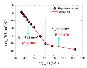
Fig. 4 The evolution of the logarithm of the conductivity *versus* the inverse of the temperature and the deduced activation energy values.
