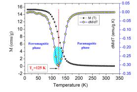
Fig. 2 Evolution of the magnetization M(T) and its derivate  $\mathrm{d}M/\mathrm{d}T$  versus the temperature for the studied system.
