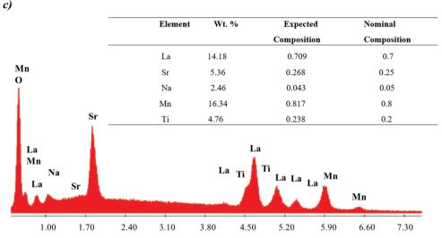
Fig. 1 X-ray diffraction results of the elaborated manganite structure (a). The scanning electron microscopy (SEM) image of the studied material (b). Results of EDAX analysis of  $La_{0.7}Sr_{0.25}Na_{0.05}Mn_{0.8}Ti_{0.2}O_3$  manganite (c).
