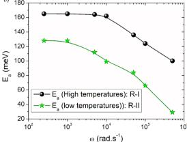
Fig. 9 Dependence of the AC conductivity on the inverse of the temperature at various frequency values (a); evolution of the activation energy *versus* the angular frequency (b).
