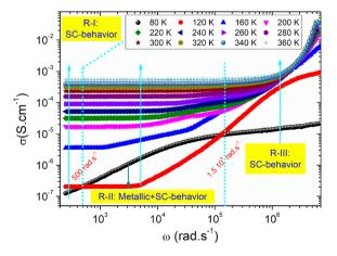
Fig. 7 Electrical conductivity spectra at various temperatures for the prepared compound.
