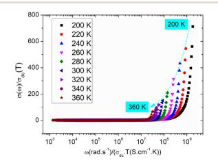
Fig. 10 Summerfield scaling of the electrical conductivity between 200 and 360 K for the studied system.
