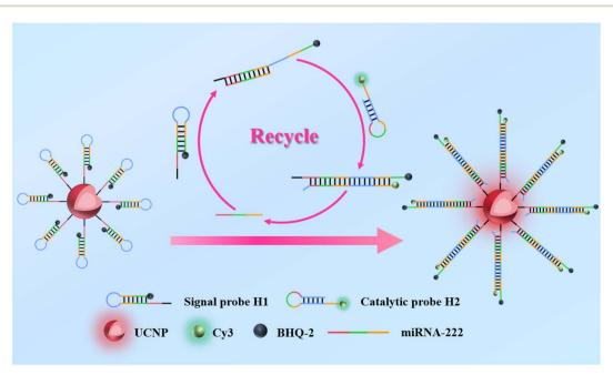
Fig. 1 Schematic diagram of the proposed biosensor for detecting miRNA.
