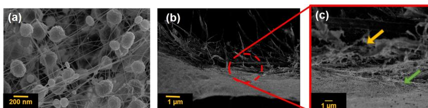
Fig. 9 (a) SEM image of the 50% w/w multimetallic silica nanohybrid incorporated CA-mat on the diaper surface, (b) and (c) SEM image of a cross section of 50% w/w multimetallic silica nanohybrid incorporated CA-mat on the diaper surface.
