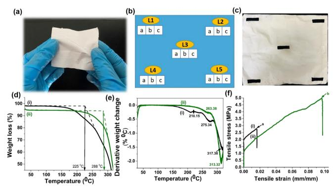
Fig. 4 (a) A digital photograph of a 50% w/w Ag-Si + Cu-Si + Co-Si-CA-mat; (b) and (c) the points where the samples were obtained to analyze band gap energies and metal composition *via* AAS analysis to confirm the homogenous distribution of each metal throughout the nanofiber mat; (d) TGA curve; (e) DTGA curve and (f) Tensile strength of (i) CA-mat, (ii) 50% w/w Ag-Si + Cu-Si + Co-Si-CA-mat.
