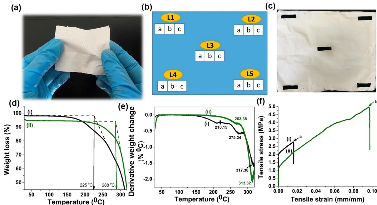
Fig. 4 (a) A digital photograph of a 50% w/w Ag-Si + Cu-Si + Co-Si-CA-mat; (b) and (c) the points where the samples were obtained to analyze band gap energies and metal composition *via* AAS analysis to confirm the homogenous distribution of each metal throughout the nanofiber mat; (d) TGA curve; (e) DTGA curve and (f) Tensile strength of (i) CA-mat, (ii) 50% w/w Ag-Si + Cu-Si + Co-Si-CA-mat.
