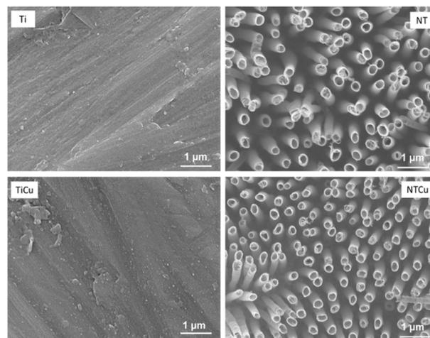
Fig. 1 Representative SEM images of different surfaces.
