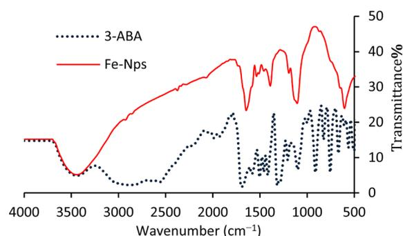
Fig. 2 Comparative FTIR spectra of 3-ABA and Fe-NPs.
