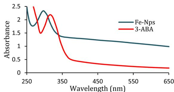
Fig. 1 Comparative UV-vis spectra of 3-ABA and Fe-NPs.
