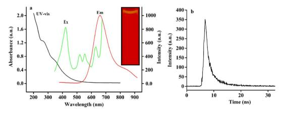
Fig. 3 (a) UV-vis absorption spectrum and fluorescence spectrum of RCDs (the illustration in the inset shows the fluorescence photos of RCDs under a 365 nm UV lamp); (b) fluorescence lifetime image of RCDs.
