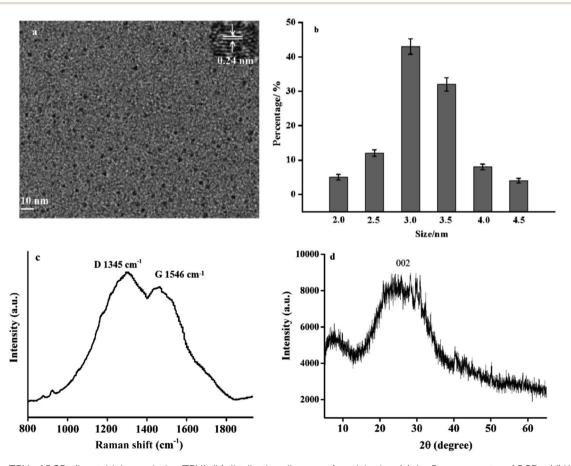
Fig. 1 (a) The TEM of RCDs (inset: high-resolution TEM); (b) distribution diagram of particle size; (c) the Raman spectra of RCDs; (d) XRD spectra of RCDs.
