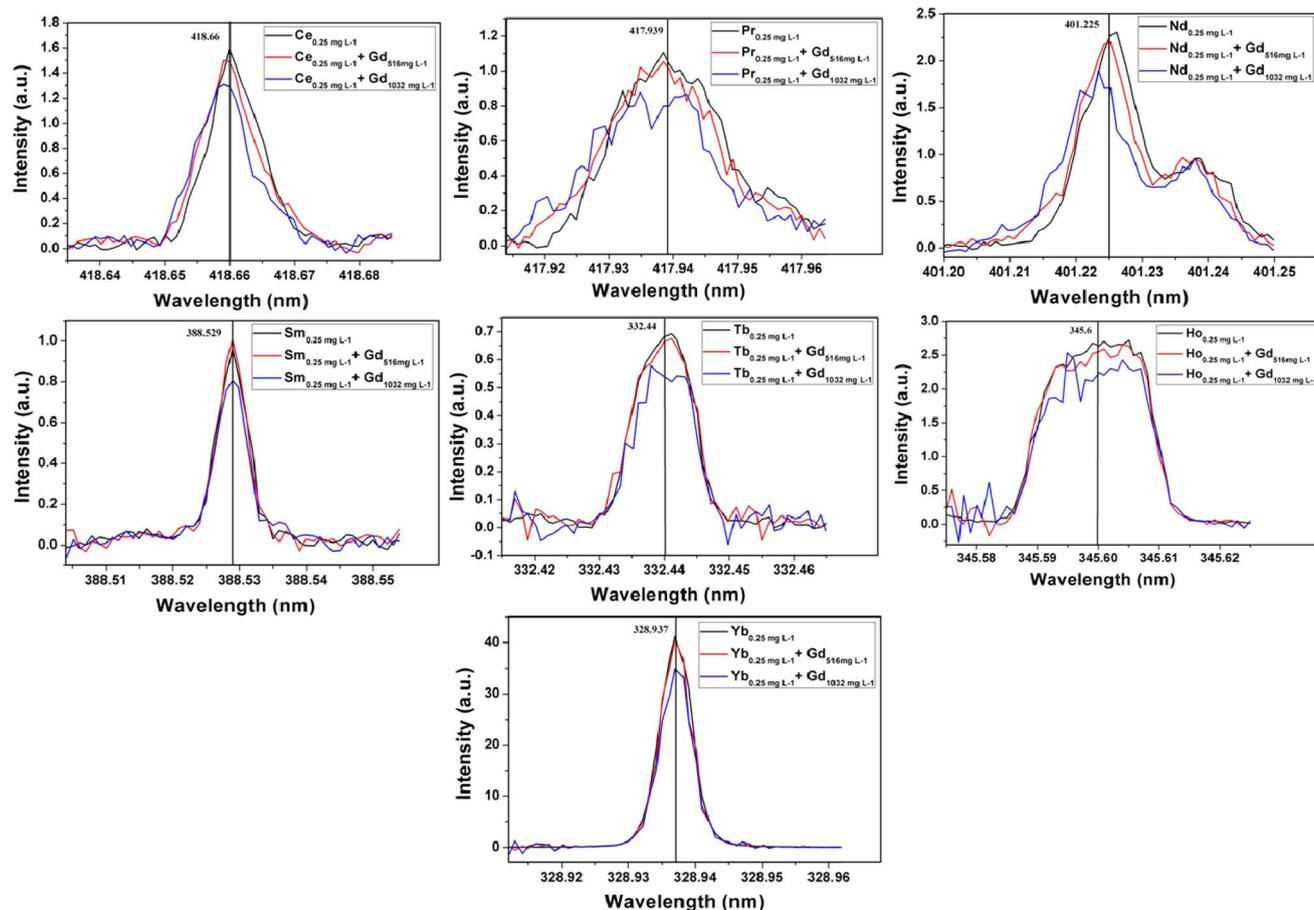
Fig. 3 Background intensity corrected emission spectra of Ce, Pr, Nd, Sm, Tb, Ho and Yb at 0.25 mg mL<sup>-1</sup> level in absence and presence of gadolinium matrix.
