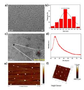
**Fig. 1** (a) TEM image of N-GQDs; (b) size distribution histogram of N-GQDs; (c) high-resolution TEM image of N-GQDs; (d) XRD patterns of N-GQDs; (e) AFM topographic image of N-GQDs; (f) AFM 3D image of N-GQDs.
