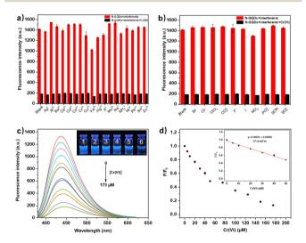
Fig. 4 (a and b) Fluorescence intensities of N-GQDs with different cations or anions in the absence/presence of  $Cr(v_1)$  (n = 3); (c) fluorescence emission spectra of N-GQDs with different concentrations of  $Cr(v_i)$  (inset: photographs of N-GQDs solution with  $Cr(v_i)$  (1–6: 0, 20, 40, 60, 80 and 100  $\mu$ M)) under 365 nm UV light; (d) the relationship between  $F/F_0$  and the concentration of  $Cr(v_1)$  (n = 3).
