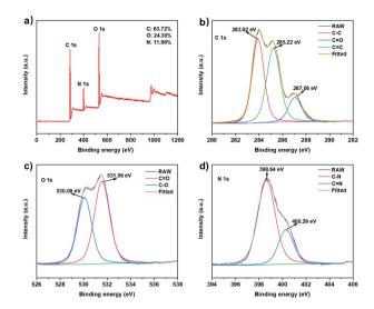
Fig. 2 XPS spectra of N-GQDs: (a) full scan; (b-d) high-resolution spectrum of C 1s, O 1s and N 1s.
