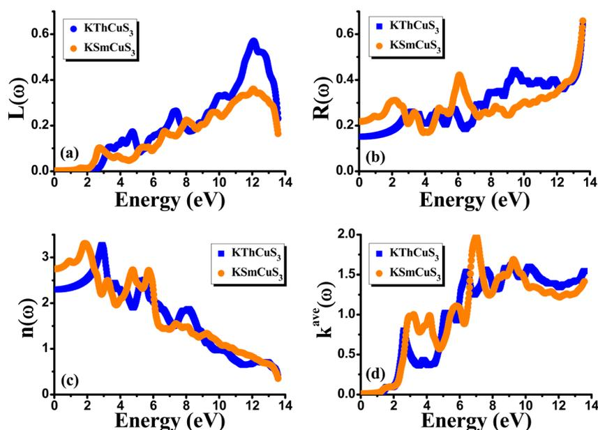
Fig. 6 The calculated (a) energy loss function (b) reflectivity (c) refractive index and (d) extinction coefficient for  $\text{KMCuS}_3$  ( $M = \text{Th}$ ,  $\text{Sm}$ ) materials.
