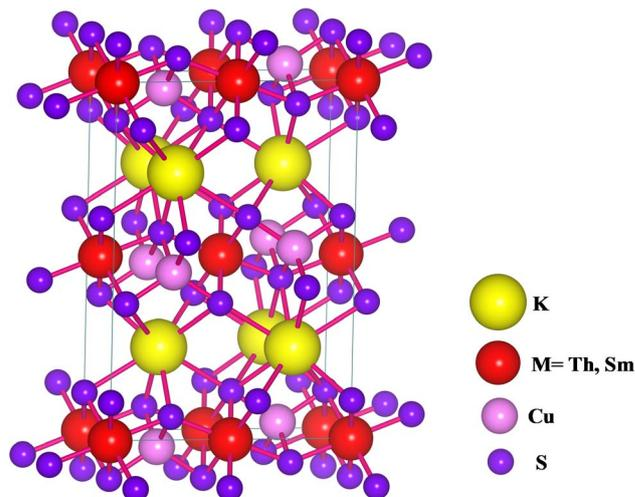
Fig. 1 The crystal structure for KMCuS<sub>3</sub> (M = Th, Sm) materials with Vesta package.
