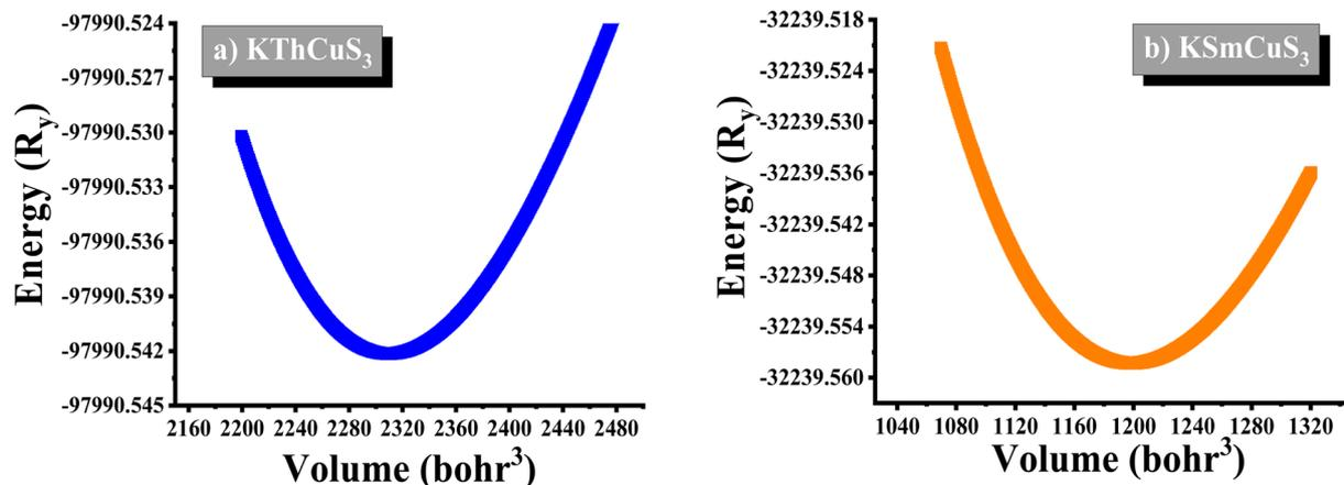
Fig. 2 The energy vs. volume optimization curves for (a) KThCuS<sub>3</sub> (b) KSmCuS<sub>3</sub> quaternary materials.
