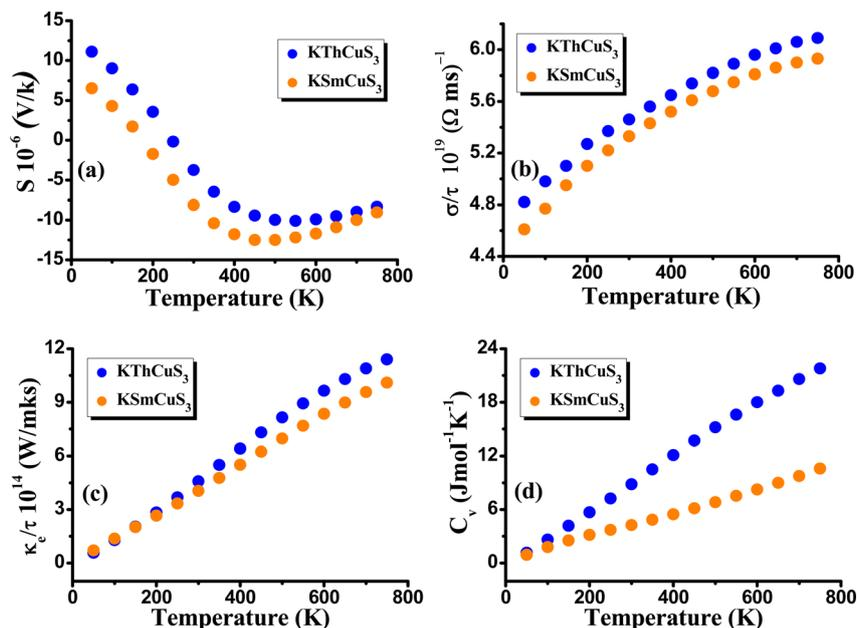
Fig. 7 The calculated (a) Seebeck coefficient (b) electrical conductivity (c) thermal conductivity and (d) specific heat capacity, for KMCuS<sub>3</sub> (M = Th, Sm) materials.
