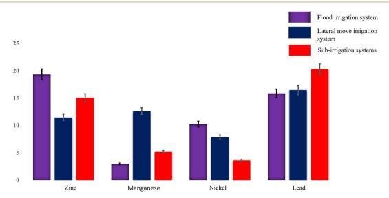
Fig. 5 Measured concentrations of zinc, manganese, nickel, and lead (shown in bars) in flood, lateral move, and sub-irrigation water systems using ESI-MPIMS
