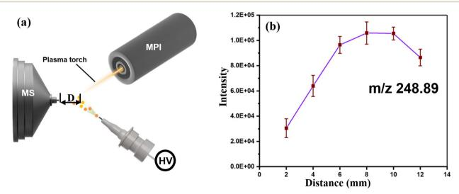
Fig. 2 System optimization. (a) A schematic representation of the system illustrating the adjustable distance (*D*) between the plasma torch and the mass spectrometer (MS) inlet. (b) Influence of the distance (*D*) on the intensity of linuron product ions (*m*/*z* 248.89). Optimal ionization is achieved at an intermediate distance. Error bars indicate the standard deviation of intensity measurements at each distance.
