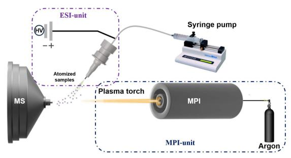
Fig. 1 Schematic diagram of the experimental setup. The system comprises two units: ESI unit for atomizing samples connected to a syringe pump to control the sample flow. MPI-unit for ionizing the atomized sample before entering the mass analyzer.
