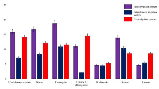
Fig. 4 Measured concentrations of 2,2,-dichroloacetamide, diuron, flumequine, 2-bromo-5-chlorophenol, norfloxacin, linuron, and linuron (shown in bars) in flood, lateral move, and sub-irrigation water systems using ESI-MPIMS.
