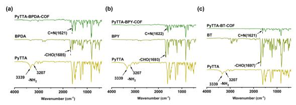
Fig. 2 FT-IR spectra of BPDA, PyTTA and PyTTA-BPDA-COF (a); BPY, PyTTA and PyTTA-BPY-COF (b); BT, PyTTA and PyTTA-BT-COF (c).
