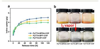
Fig. 4 Iodine adsorption behavior of PyTTA-BPDA-COF, PyTTA-BPY-COF, and PyTTA-BT-COF (a) and their color changes (b).
