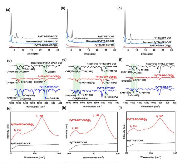
Fig. 6 PXRD spectra of PyTTA-BPDA-COF (a), PyTTA-BPY-COF (b), PyTTA-BT-COF (c) before and after I<sub>2</sub> adsorption and desorption. FT-IR spectra spectroscopy of PyTTA-BPDA-COF (d), PyTTA-BPY-COF (e), PyTTA-BT-COF (f) before and after I<sub>2</sub> adsorption and desorption. Raman spectra of PyTTA-BPDA-COF (g), PyTTA-BPY-COF (h), PyTTA-BT-COF (i) before and after I<sub>2</sub> adsorption and desorption.
