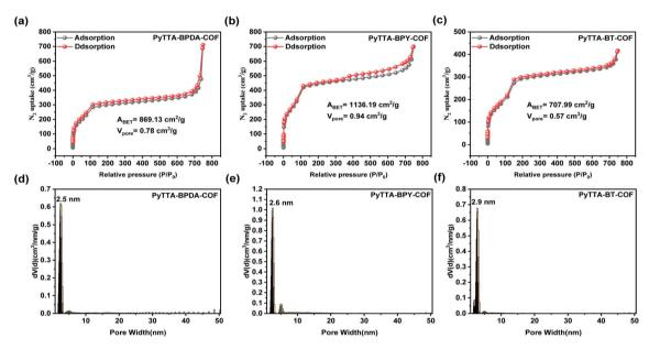
Fig. 3  $N_2$  adsorption isotherms and pore size distribution of PyTTA-BPDA-COF (a and d), PyTTA-BPY-COF (b and e), and PyTTA-BT-COF (c and f).
