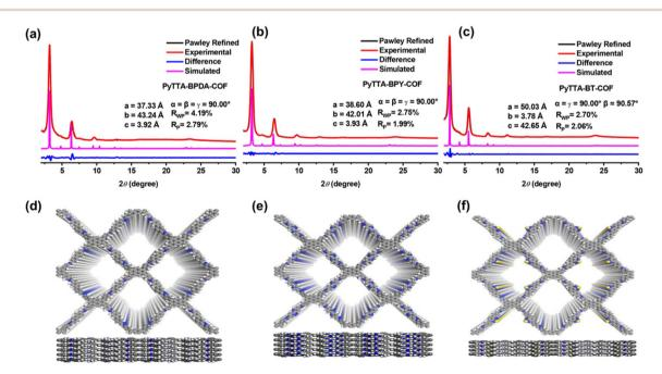
Fig. 1 PXRD profiles of PyTTA-BPDA-COF (a), PyTTA-BPY-COF (b), PyTTA-BT-COF (c) for experimentally observed, Pawley refined, calculated for the AA stacking model, and the difference between experimental and calculated data.
