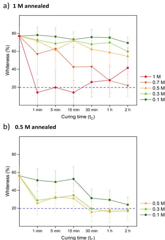
Fig. 3 The whiteness change over time of (a) 1 M annealed and (b) 0.5 M annealed samples when cured in different concentrations of KBr. The blue dashed line represents the whiteness of the blank. The error bars represent the standard deviations of triplets.
