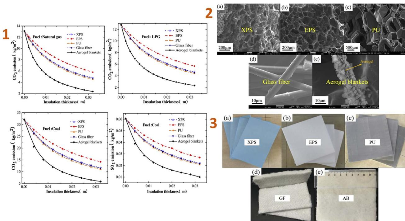
Fig. 1 (1) Effect *versus* the thickness on CO<sub>2</sub> and SO<sub>2</sub> emissions of five insulation materials; (2) SEM images of five types of insulation materials: (a) XPS, (b) EPS, (c) PU foam, (d) GF, (e) aerogel blankets; (3) optical image of five types of insulation materials: (a) XPS, (b) EPS, (c) PU foam, (d) GF, (e) aerogel blankets. This figure has been adapted/reproduced from ref. 129 with permission from Elsevier under the license number 5823621056830, copyright 2024.
