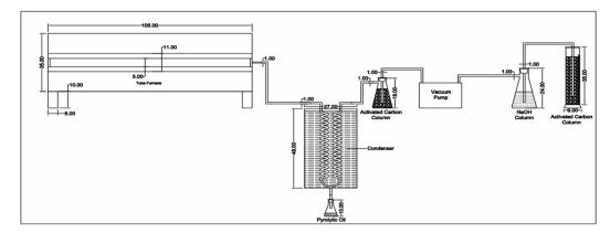
Fig. 1 Schematic diagram of pyrolytic oil set-up (ref. 50).
