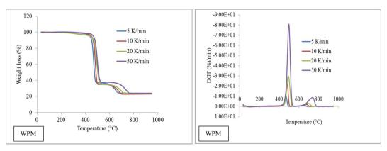
Fig. 2 Plots of TGA and DTG of WPM.
