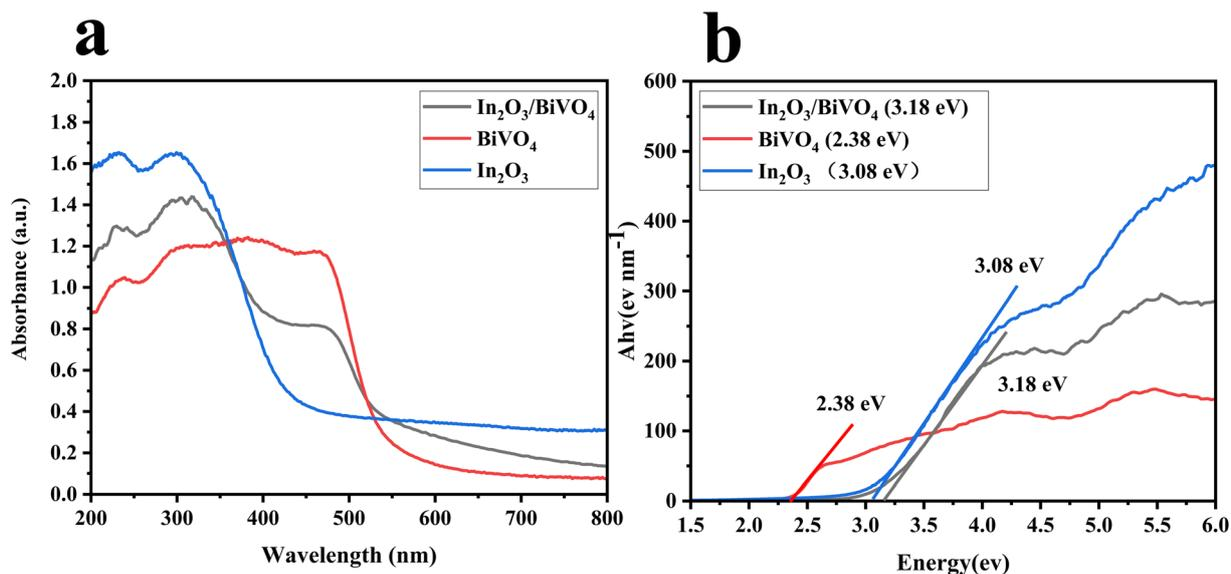
Fig. 7 (a) The UV absorption spectra of  $\text{In}_2\text{O}_3$ ,  $\text{BiVO}_4$  and  $\text{In}_2\text{O}_3/\text{BiVO}_4$ . (b) The optical band-gap fitting curve of  $\text{In}_2\text{O}_3$ ,  $\text{BiVO}_4$  and  $\text{In}_2\text{O}_3/\text{BiVO}_4$ .
