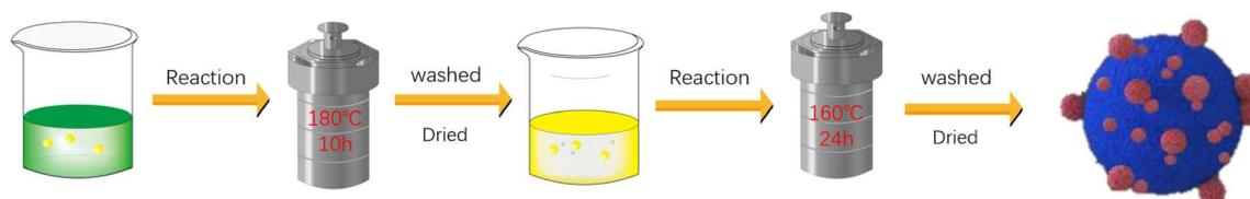
Fig. 1 In<sub>2</sub>O<sub>3</sub>/BiVO<sub>4</sub> preparation procedure.
