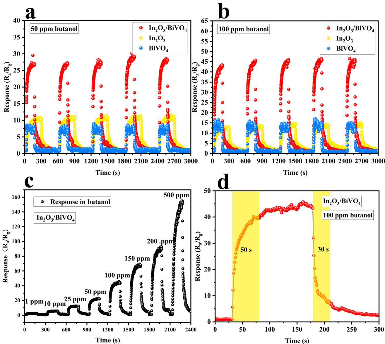
Fig. 10 (a and b) Repeatability test responses of  $\text{In}_2\text{O}_3$ ,  $\text{BiVO}_4$  and  $\text{In}_2\text{O}_3/\text{BiVO}_4$  to butanol at 50 ppm and 100 ppm. (c) Response of  $\text{In}_2\text{O}_3/\text{BiVO}_4$  to butanol at different concentrations. (d) Adsorption–desorption time of  $\text{In}_2\text{O}_3/\text{BiVO}_4$  at 100 ppm butanol.
