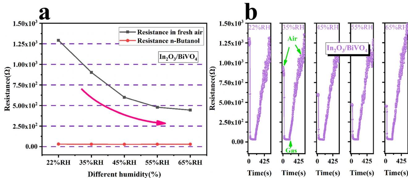
Fig. 11 (a) Resistance of In<sub>2</sub>O<sub>3</sub>/BiVO<sub>4</sub> in butanol and air at different humidities. (b) Resistance of In<sub>2</sub>O<sub>3</sub>/BiVO<sub>4</sub> for 100 ppm butanol at different humidities.
