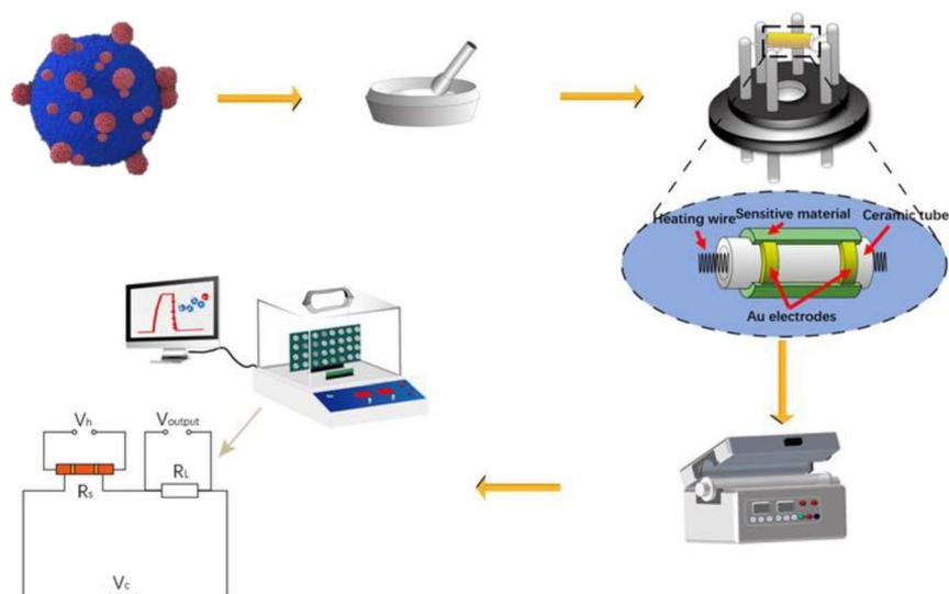
Fig. 2 Sensor preparation process and test process.
