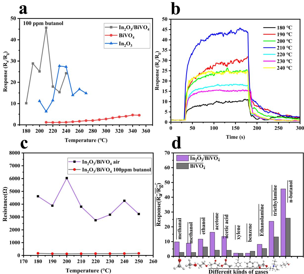
Fig. 9 (a) Response of In<sub>2</sub>O<sub>3</sub>, BiVO<sub>4</sub> and In<sub>2</sub>O<sub>3</sub>/BiVO<sub>4</sub> to different temperatures at 100 ppm butanol. (b) Response of In<sub>2</sub>O<sub>3</sub>/BiVO<sub>4</sub> at different temperatures to 100 ppm butanol. (c) Resistance of In<sub>2</sub>O<sub>3</sub>/BiVO<sub>4</sub> in the air and butanol at different temperatures. (d) Selectivity test of BiVO<sub>4</sub> and In<sub>2</sub>O<sub>3</sub>/BiVO<sub>4</sub>.
