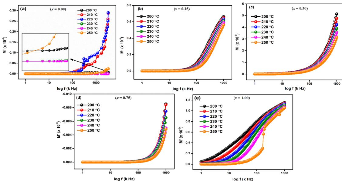
Fig. 9 Frequency dependent real part of modulus ( $M'$ ) of  $\text{LaMn}_{1-x}\text{Fe}_x\text{O}_3$  ceramics.
