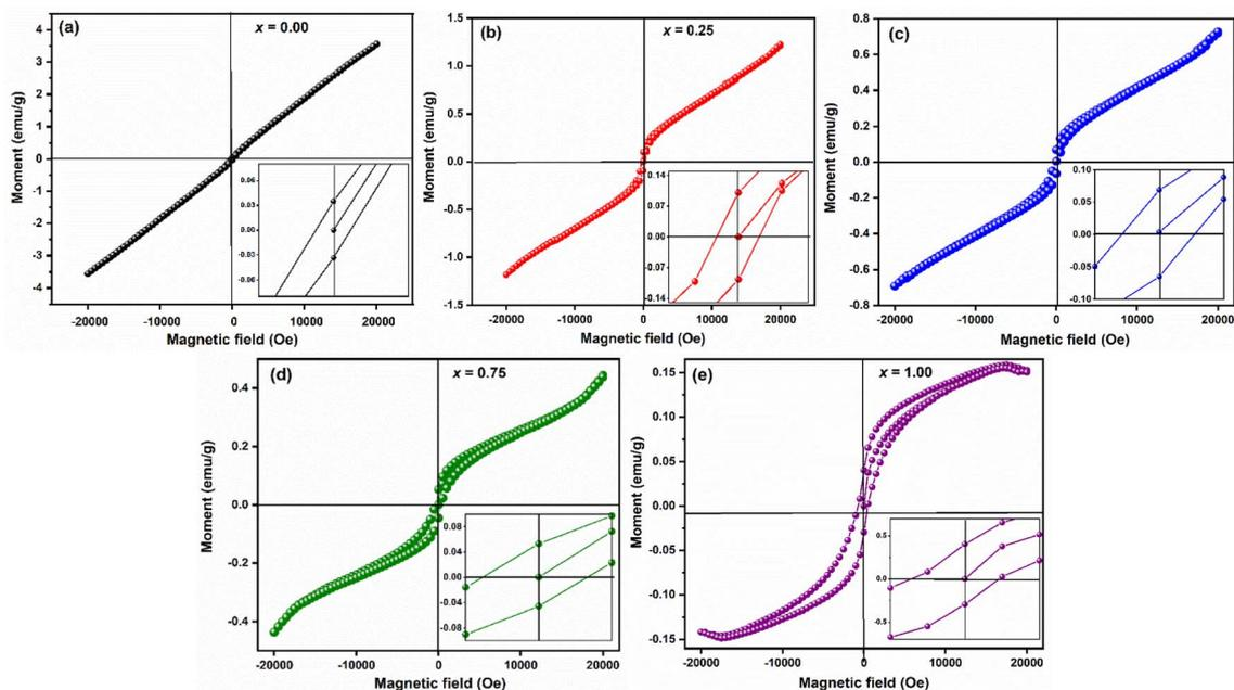
Fig. 14 Room-temperature M – H loop of  $\text{LaMn}_{1-x}\text{Fe}_x\text{O}_3$  ceramics.
