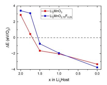
Fig. 5 Calculated formation energy for the reaction of  $O_2$  in  $Li_2MnO_3$  and  $Li_2MnO_{2.75}F_{0.25}$  during delithiation.
