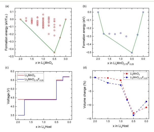
Fig. 2 The formation energies (a)  $\text{Li}_2\text{MnO}_3$  and (b)  $\text{Li}_2\text{MnO}_{2.75}\text{F}_{0.25}$ . (c) The voltage profiles of  $\text{Li}_2\text{MnO}_3$  and  $\text{Li}_2\text{MnO}_{2.75}\text{F}_{0.25}$ . (d) The volume change of  $\text{Li}_2\text{MnO}_3$  and  $\text{Li}_2\text{MnO}_{2.75}\text{F}_{0.25}$ .
