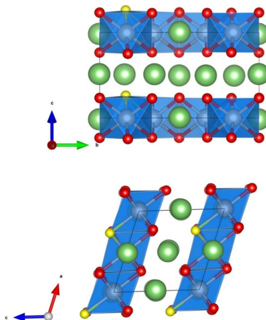
Fig. 1 The crystal structure of  $\text{Li}_2\text{MnO}_{2.75}\text{F}_{0.25}$ . The Li and O atoms are denoted by green and red spheres, respectively. The substituted O atom by F is shown as a yellow sphere. The  $\text{MnO}_6$  octahedra are highlighted in blue.
