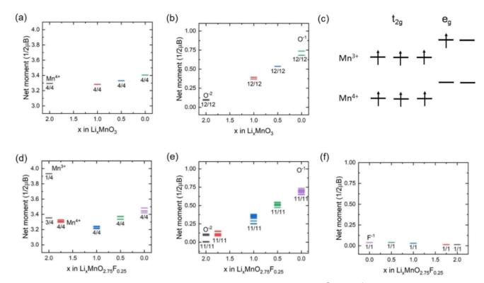
Fig. 4 Magnetic moment variation of (a) Mn and (b) O in  $\text{Li}_2\text{MnO}_3$ . (c) Schematic diagrams of  $\text{Mn}^{3+}$  and  $\text{Mn}^{4+}$ . Corresponding magnetic moment variation of (d) Mn, (e) O and (f) F in  $\text{Li}_2\text{MnO}_{2.75}\text{F}_{0.25}$ .
