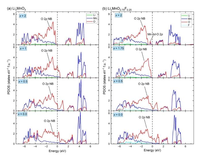
Fig. 3 The density of states for (a)  $\text{Li}_x \text{MnO}_3$  and (b)  $\text{Li}_x \text{MnO}_{2.75} \text{F}_{0.25}$ . The non-bonding O 2p states is denoted as "O 2p NB", the hybridized Mn 3d–O 2p states is denoted as "Mn 3d–O 2p".
