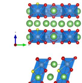
Fig. 1 The crystal structure of  $Li_2MnO_{2.75}F_{0.25}$ . The Li and O atoms are denoted by green and red spheres, respectively. The substituted O atom by F is shown as a yellow sphere. The MnO<sub>6</sub> octahedra are highlighted in blue.
