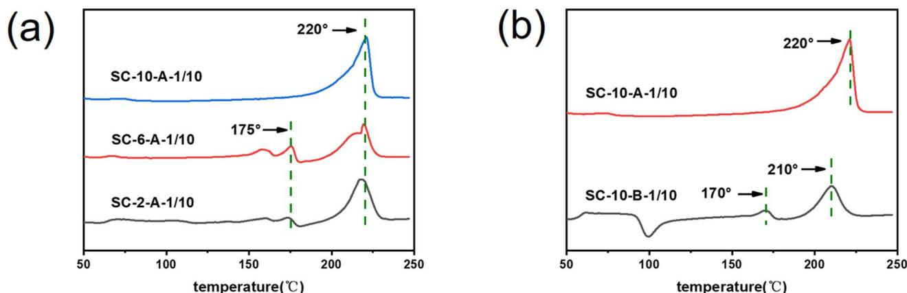
Fig. 5 DSC images of sc-PLA nano-microspheres: (a) different concentrations: 2 wt%, 6 wt%, 10 wt%, (b) different treatments: stationary, stirred.
