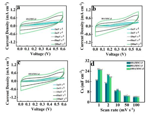
CVs for (a) 60AMSCs3, (b) 80AMSCs3, (c) 100AMSCs3 at 1–100 mV s<sup>-1</sup> and (d) corresponding capacitance derived from CV profiles.
