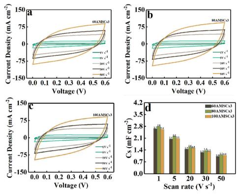
Fig. 8 CVs for (a) 60AMSCs3, (b) 80AMSCs3, (c) 100AMSCs3 at 1–50 V s<sup>-1</sup> and (d) corresponding capacitance derived from CV profiles.
