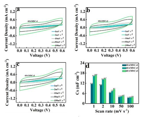
Fig. 4 CVs for (a) 60AMSCs1, (b) 60AMSCs2, (c) 60AMSCs3 at 1–100 mV s<sup>-1</sup> and (d) corresponding capacitance derived from CV profiles.
