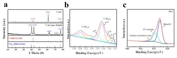
Fig. 3 (a) XRD profiles, and XPS spectra of (b) V 2p and (c) O 1s, for V-MS after WEDM.
