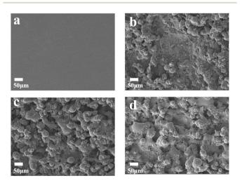
Fig. 2 SEM images of V-MS (a) before vanadium plate processing and integrated electrode at different processing voltages (b) 60 V; (c) 80 V; (d) 100 V.
