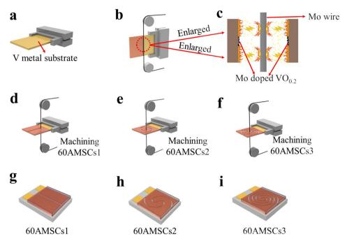
Fig. 1 (a) Untreated V-MS and (b) V-MS during WEDM and (c) enlarged electric discharge channel for generating Mo doped  $VO_{0.2}$  particles during WEDM and (d–i) manufacturing process of Mo doped  $VO_{0.2}$  PC-MSCs devices with different modes.
