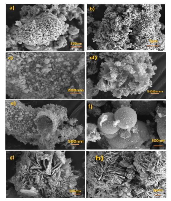
Fig. 3 FE-SEM images (a and b) for MOFP1, (c-e) for MOFP2, and (f-h) for MOFP3 at different magnification scales.
