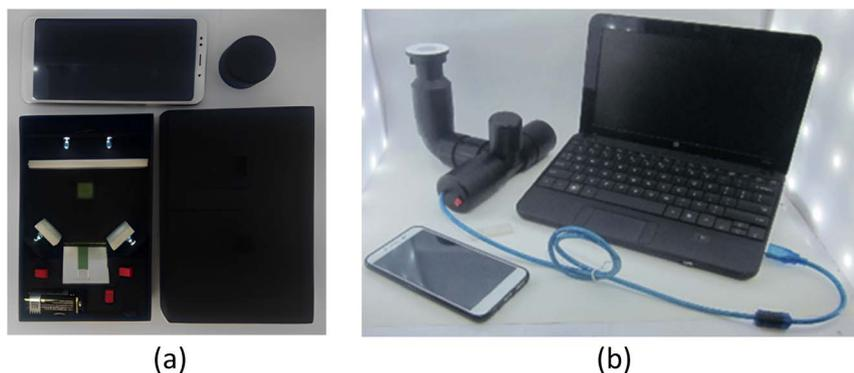
Fig. 8 Micro-studios for controlling light; (a) cuboid and (b) T-shape models.
