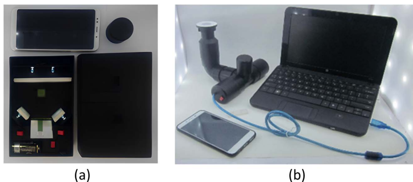
Fig. 8 Micro-studios for controlling light; (a) cuboid and (b) T-shape models.
