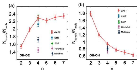
Fig. 5 Number of hydrogen bonds between hydroxy hydrogen and (a) ether oxygen (OH–OE) and (b) hydroxy oxygen (OH–OH) per PEG molecule as function of oligomer size  $n$  using the original and charge modified GAFF force field.
