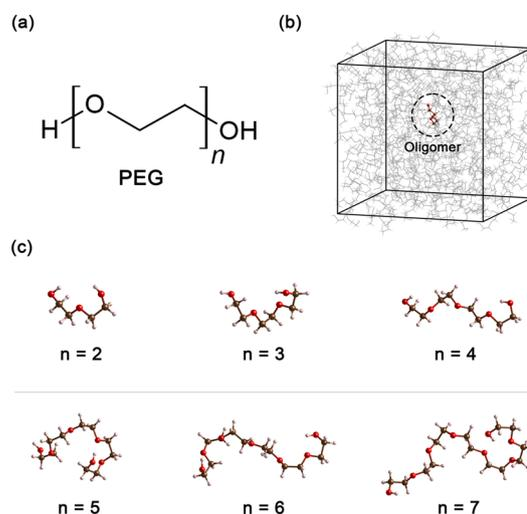
**Fig. 1** (a) Chemical formula of PEG200, where  $n$  signifies the number of repeating ethylene oxide units. (b) Cubic unit cell in MD simulation, containing an oligomer molecule at its center for presenting neat PEG oligomer with size  $n$  (c) snapshot of six oligomers obtained from the MD simulation, illustrating the increase in the number of repeating units,  $n$  from 2 to 7.
