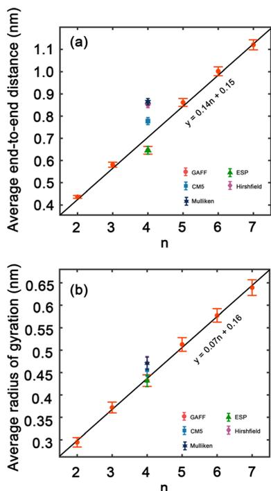
**Fig. 3** (a) Average end-to-end distance of ethylene glycol oligomers of hydroxy oxygen atoms and (b) average radii of gyration of ethylene glycol oligomers,  $\leq 120^\circ$  in PEG200 with included standard deviations. The values from different charge models are included for comparison. Solid lines are linear fits.
