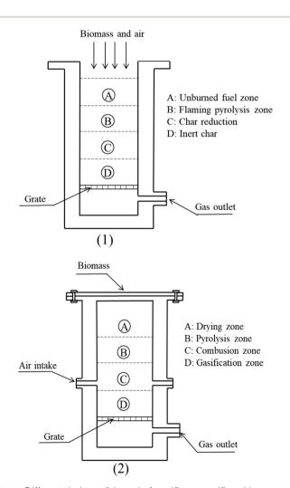
Fig. 1 Different designs of downdraft gasifiers: a gasifier with open top (1) and a gasifier with closed top (2).
