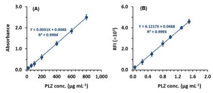
Fig. 6 Calibration curves for the determination of PLZ by MW-PM (A) and MW-FL (B) assays via its reaction with NBD-F probe. RFI is the relative fluorescence intensity. Each point is the average of 5 replicate measurements, and the presented error bars are the standard deviations of the reading at 95% confidence. Linear fitting equations with their corresponding determination coefficients ( $R^2$ ) are given on the lines.
