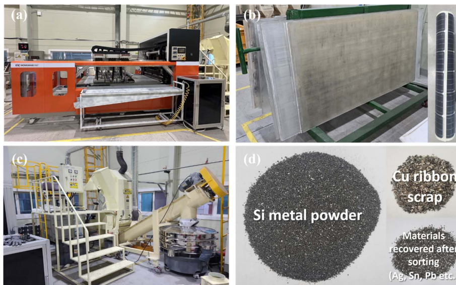
Fig. 3 Process overview of hot-knife, crushing, and sorting, (a) hot-knife equipment, (b) recovered front cover glass and curled Si solar cells after the hot-knife process, (c) crushing and sorting process, and (d) final products after whole recycling processes.
