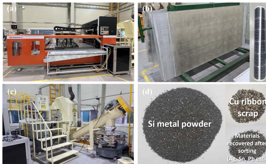
Fig. 3 Process overview of hot-knife, crushing, and sorting, (a) hot-knife equipment, (b) recovered front cover glass and curled Si solar cells after the hot-knife process, (c) crushing and sorting process, and (d) final products after whole recycling processes.
