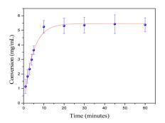
Fig. 4 Time-course of the conversion of 1a (0.14 mmol) into 2a in toluene/water (2 mL: 2 mL) at room temperature with 1 mol% of C1.
