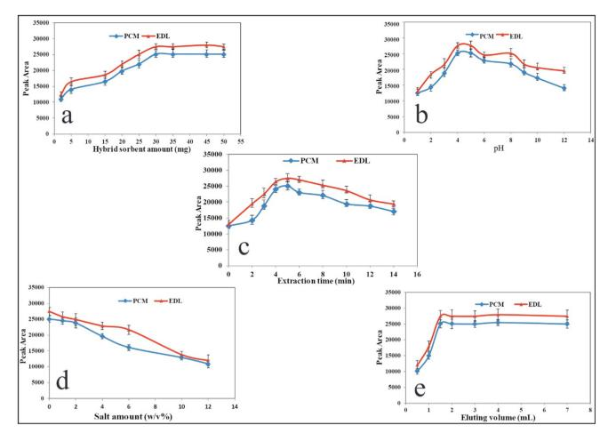
Fig. 7 Variables affecting the performance of US-A-MDMSPE-HPLC-UV. Effect of (a) the dosage of CQDs/ZIF-90/PVP/Fe<sub>3</sub>O<sub>4</sub>, (b) pH, (c) extraction time, (d) salt amount and (e) volume of desorbing agents. Other conditions: PCM and EDL at a concentration level of 200 ng mL<sup>-1</sup> for every drug, sample volume of 5.0 mL, desorption time 4.0 min.
