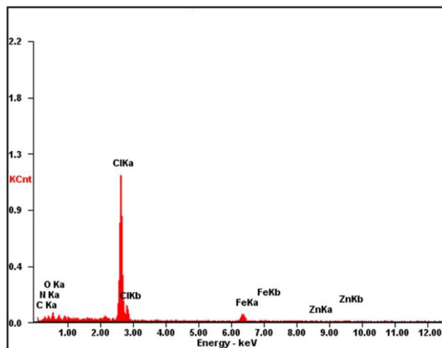
Fig. 5 Energy-dispersive X-ray spectrum of CQDs/ZIF-90/PVP/Fe<sub>3</sub>O<sub>4</sub>.
