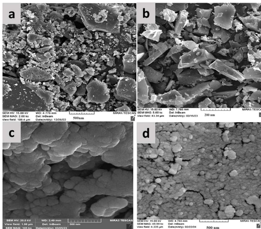
Fig. 6 Field-emission scanning electron microscopic (FE-SEM) images of (a) CQDs, (b) CQDs/ZIF-90, (c) CQDs/ZIF-90/PVP and (d) CQDs/ZIF-90/PVP/Fe<sub>3</sub>O<sub>4</sub>.
