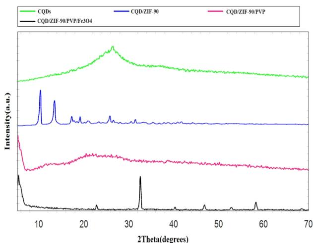
Fig. 4 X-ray diffraction patterns of CQDs, CQDs/ZIF-90, CQDs/ZIF-90/PVP and CQDs/ZIF-90/PVP/Fe<sub>3</sub>O<sub>4</sub>.
