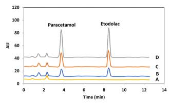
Fig. 8 Different HPLC-UV chromatograms of the target drugs of PCM and EDL in human plasma: (A) blank; human plasma samples spiked with the concentration level of each drug at (B) 100 ng mL<sup>-1</sup>, (C) 200  ${\rm ng}\ {\rm mL}^{-1}\ {\rm and}\ ({\rm D})\ 400\ {\rm ng}\ {\rm mL}^{-1}$
