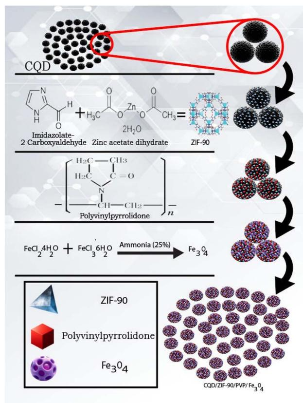
Fig. 1 Schematic diagram of the synthesis routes of CQDs/ZIF-90/PVP/Fe<sub>3</sub>O<sub>4</sub>.
