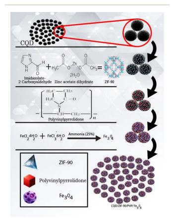
Fig. 1 Schematic diagram of the synthesis routes of CQDs/ZIF-90/  $PVP/Fe_3O_4$ .
