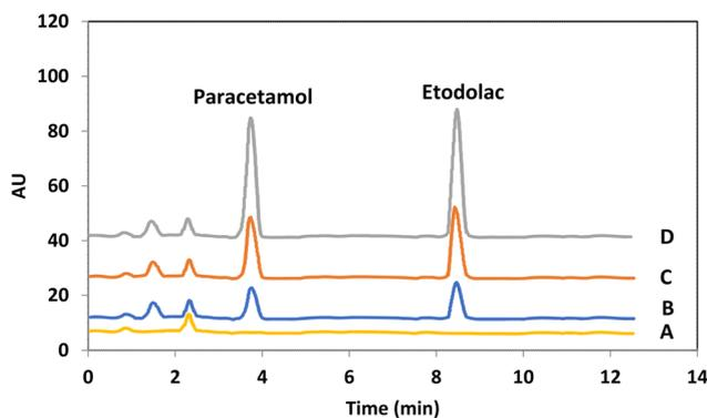
Fig. 8 Different HPLC–UV chromatograms of the target drugs of PCM and EDL in human plasma: (A) blank; human plasma samples spiked with the concentration level of each drug at (B) 100 ng mL<sup>-1</sup>, (C) 200 ng mL<sup>-1</sup> and (D) 400 ng mL<sup>-1</sup>.
