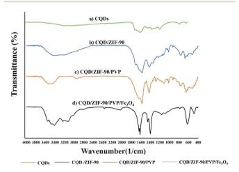
Fig. 3 Fourier transform infrared spectra of (a) CQDs, (b) CQDs/ZIF-90, (c) CQDs/ZIF-90/PVP and (d) CQDs/ZIF-90/PVP/Fe $_3$ O $_4$ .
