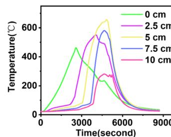
Fig. 3 Temperature curve when smoldering occurs.
