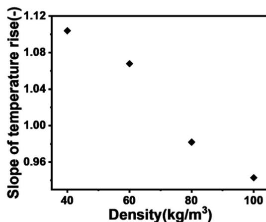
Fig. 10 Temperature rise rate as a constructor of density, provided by the fitted curve in Fig. 5.
