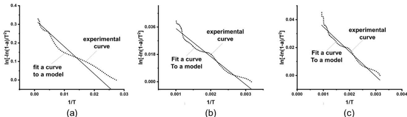
Fig. 7 First-order kinetic correlation analysis curves for calcium alginate fibers: (a)  $\beta = 10 \text{ }^\circ\text{C min}^{-1}$ ; (b)  $\beta = 15 \text{ }^\circ\text{C min}^{-1}$ ; (c)  $\beta = 20 \text{ }^\circ\text{C min}^{-1}$ .
