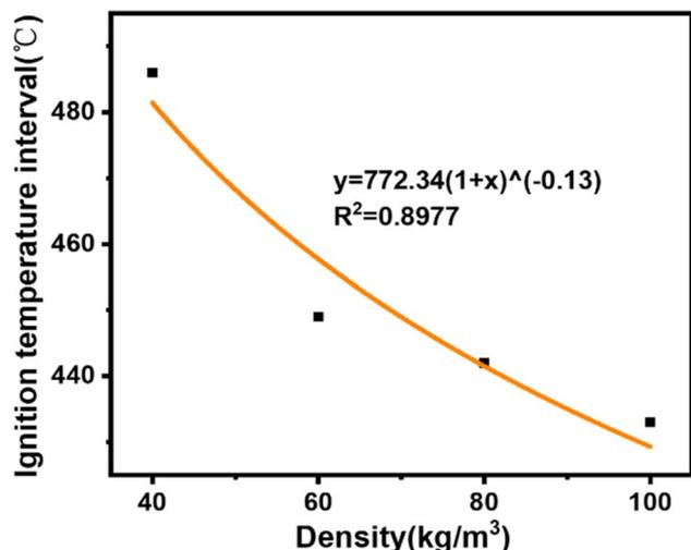
Fig. 5 Density-temperature curve of calcium alginate fiber.
