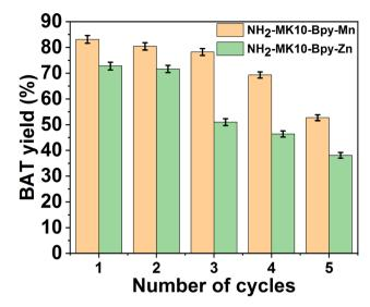
Fig. 6 Reusability of NH<sub>2</sub>-MK10-Bpy-Zn and NH<sub>2</sub>-MK10-Bpy-Mn catalysts in the transesterification of EAA under optimum conditions.
