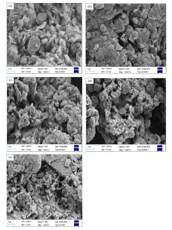
Fig. 4 SEM images of (a) MK10, (b) NH<sub>2</sub>-MK10, (c) NH<sub>2</sub>-MK10-Bpy, (d) NH<sub>2</sub>-MK10-Bpy-Zn and (e) NH<sub>2</sub>-MK10-Bpy-Mn.
