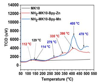
Fig. 2 NH<sub>3</sub>-TPD profiles of MK10, NH<sub>2</sub>-MK10-Bpy-Zn and NH<sub>2</sub>-MK10-Bpy-Mn.
