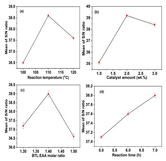
Fig. 5 Plots of mean of the S/N ratio as a function of (a) temperature, (b) catalyst amount, (c) the BTL: EAA molar ratio and (d) reaction time.
