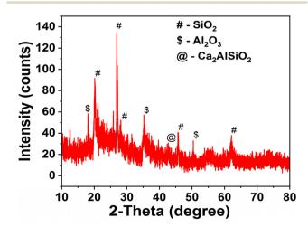
Fig. 1 XRD pattern of the MK10 sample.
