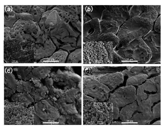
Fig. 3 The SEM images of the anisotropic cellulose/SiO<sub>2</sub> aerogel composite biomimetic thermal control material, (a) CS-1.0, (b) CS-2.5, (c) CS-5.0 and (d) CS-10.0.
