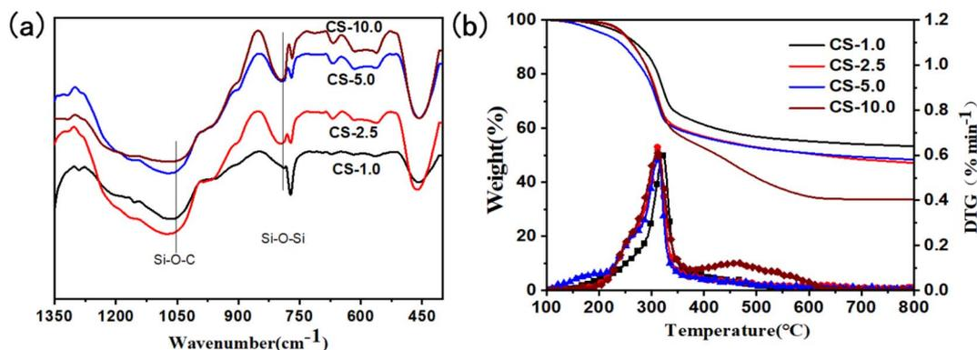
Fig. 4 The FT-IR spectrums (a), and the TG curves (b) of the anisotropic cellulose/SiO<sub>2</sub> composite biomimetic thermal control materials.
