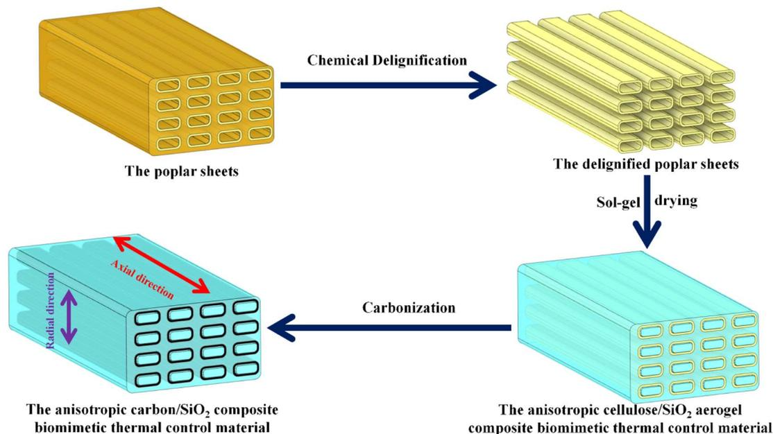
Fig. 1 Illustration of fabrication process for the of the anisotropic carbon/SiO<sub>2</sub> composite biomimetic thermal control material.
