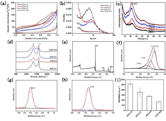
Fig. 6  $N_2$  adsorption and desorption isotherm (a), pore size distribution (b), XRD (c), and Raman spectrum (d) of the anisotropic carbon/SiO<sub>2</sub> composite biomimetic thermal control materials, the full spectrum (e), high resolution C 1s (f), high resolution Si 2p (g) and O 1s (h) XPS spectra of the ACS-2.5 composite biomimetic thermal control materials, the density (i) of the anisotropic carbon/SiO<sub>2</sub> composite biomimetic thermal control materials.
