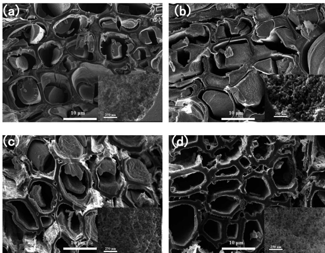
Fig. 5 The SEM images of the anisotropic carbon/SiO<sub>2</sub> aerogel composite biomimetic thermal control materials, (a) ACS-1.0, (b) ACS-2.5, (c) ACS-5.0 and (d) ACS-10.0.
