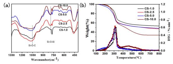
Fig. 4 The FT-IR spectrums (a), and the TG curves (b) of the anisotropic cellulose/SiO<sub>2</sub> composite biomimetic thermal control materials.
