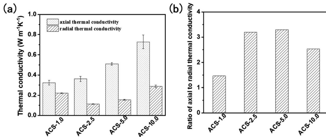
Fig. 7 Thermal conductivity (a) and the ratio of the axial thermal conductivity to radial thermal conductivity (b) of the anisotropic carbon/SiO<sub>2</sub> composite biomimetic thermal control materials.
