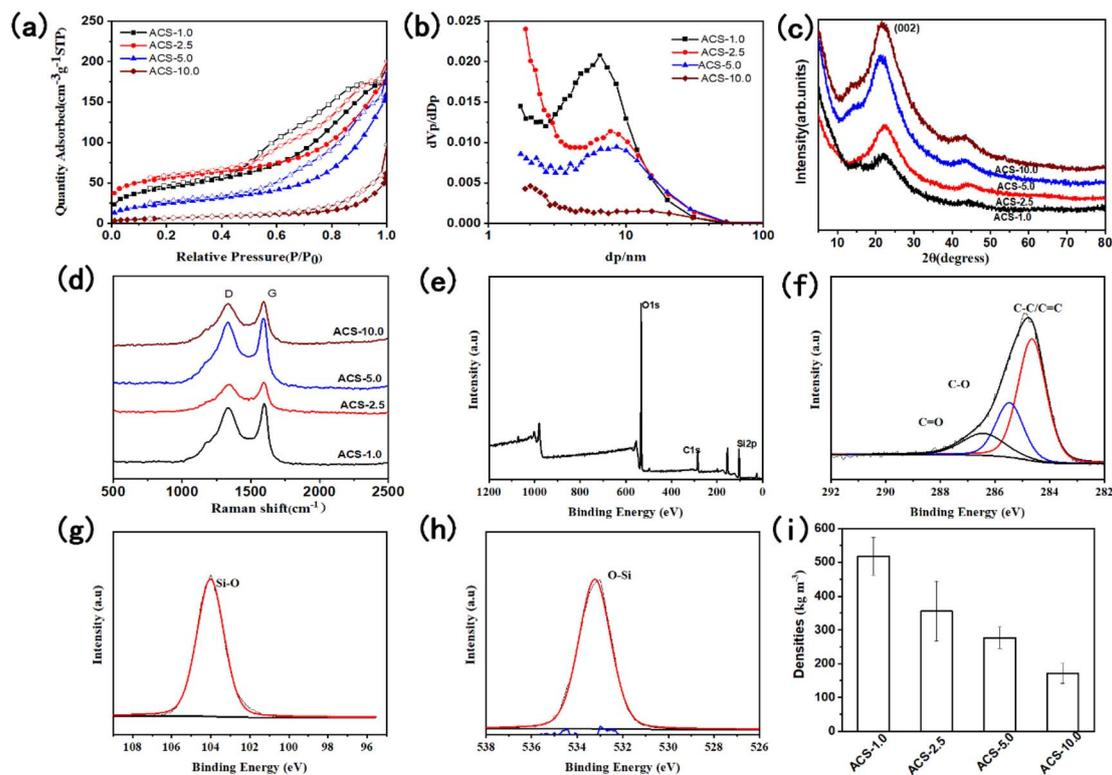
Fig. 6  $N_2$  adsorption and desorption isotherm (a), pore size distribution (b), XRD (c), and Raman spectrum (d) of the anisotropic carbon/SiO<sub>2</sub> composite biomimetic thermal control materials, the full spectrum (e), high resolution C 1s (f), high resolution Si 2p (g) and O 1s (h) XPS spectra of the ACS-2.5 composite biomimetic thermal control materials, the density (i) of the anisotropic carbon/SiO<sub>2</sub> composite biomimetic thermal control materials.
