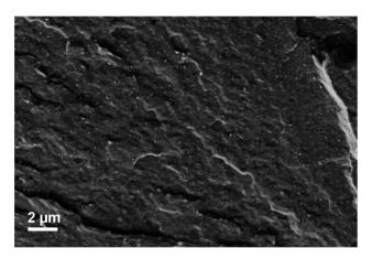
**Fig. 1** SEM micrograph of the cryofractured surface of PBAT/1% MWCNT nanocomposites.
