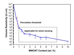
**Fig. 4** Electrical volume resistivity of PBAT/MWCNT nanocomposites *versus* MWCNT content.
