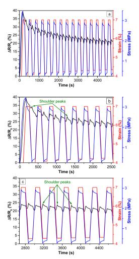
Fig. 7 Cyclic-strain test of PBAT/3% MWCNT nanocomposites with 7% mechanical strain and 15 cycles: (a) wide regime (b) first half of the test and (c) second half of the test.
