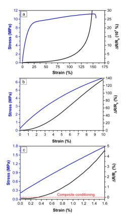
Fig. 5 Stress-strain behaviour and the relative resistance change ( $\Delta R/R_0$ ) of PBAT/3% MWCNT nanocomposites: (a) overview, (b) narrower regime – up to 10% strain, (c) narrowest regime – up to 1.5% strain.
