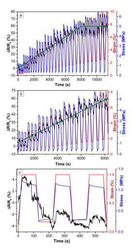
Fig. 6 Cyclic-strain test of PBAT/3% MWCNT nanocomposites with increasing mechanical strain: (a) wide regime (b) closer regime up to 8% strain and (c) closest regime up to 1% strain.
