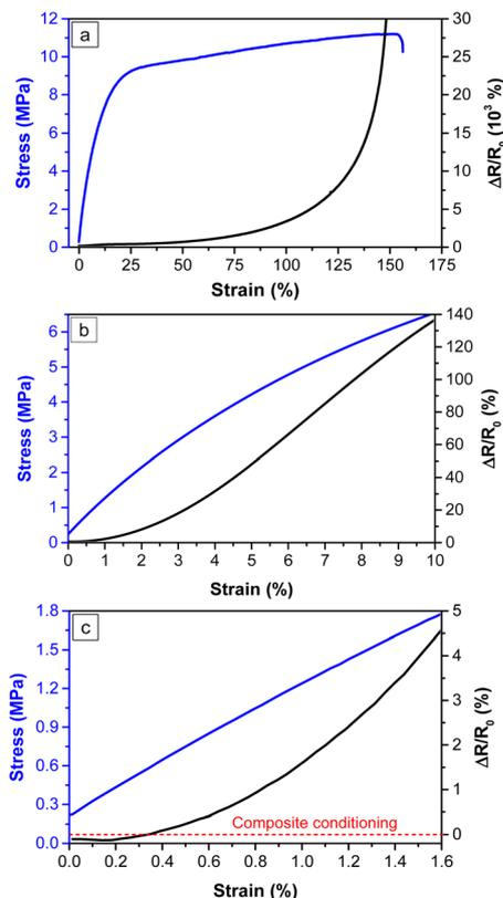
Fig. 5 Stress–strain behaviour and the relative resistance change ( $\Delta R/R_0$ ) of PBAT/3% MWCNT nanocomposites: (a) overview, (b) narrower regime – up to 10% strain, (c) narrowest regime – up to 1.5% strain.
