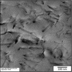
Fig. 2 TEM micrographs of PBAT/3% MWCNT nanocomposites under different magnifications.
